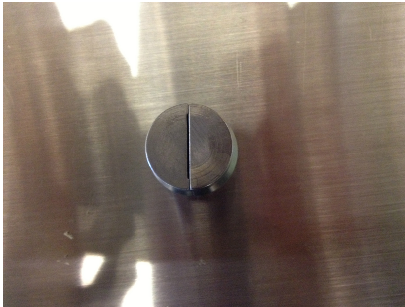
Figure 3.2: Slots made up of two "half-circles" used to simulate fracture.
