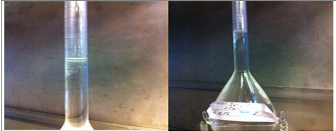
Fig. 50 Formed emulsion with presence of some fines during imbibition test with SK_C core
