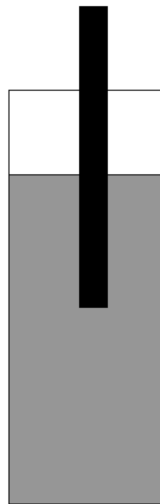
Figure 2.3 - A picture showing reduced annulus mud height after losses [8]
