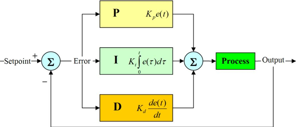
Figure 29 Block diagram of a PID-controller. Figure is taken from [27].
