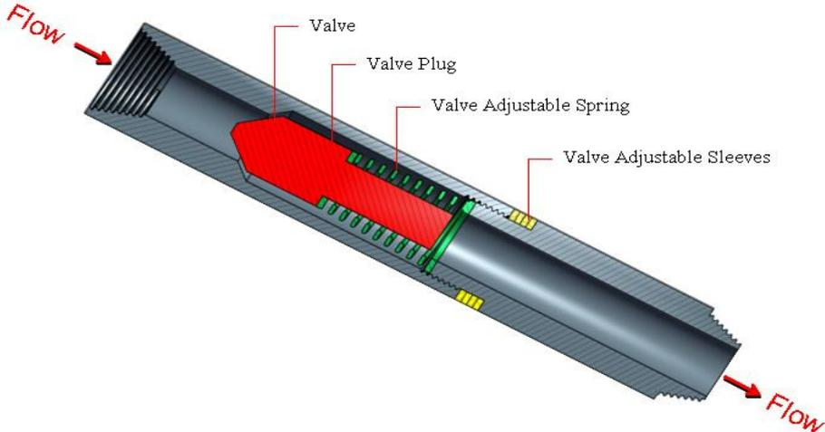
**Figure 32** Schematic drawing of a Flow Stop Sub. Figure is taken from Baker Hughes [28].
