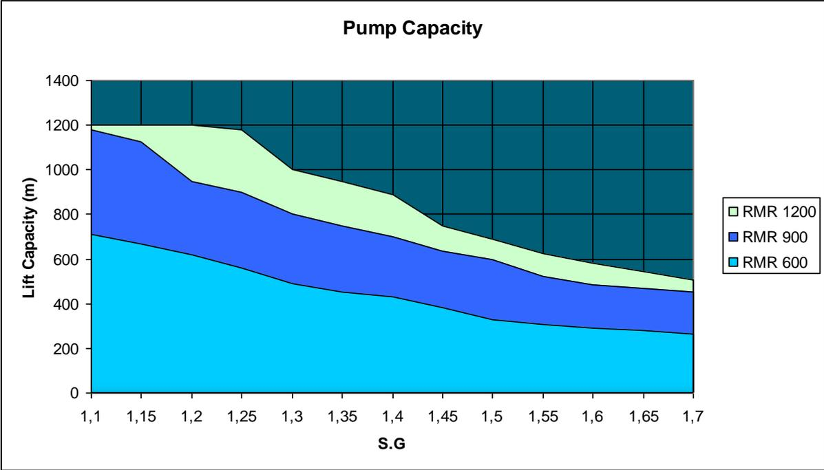
Figure 37 Pump efficiency graph for RMR<sup>®</sup>600, RMR<sup>®</sup>900 and RMR<sup>®</sup>1200. For presentation purpose only. Data is taken from AGR.
