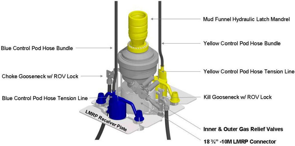
**Figure 20** Modified “Built for Purpose” Lower Marine Riser Package schematic. Figure is taken from ORS.
