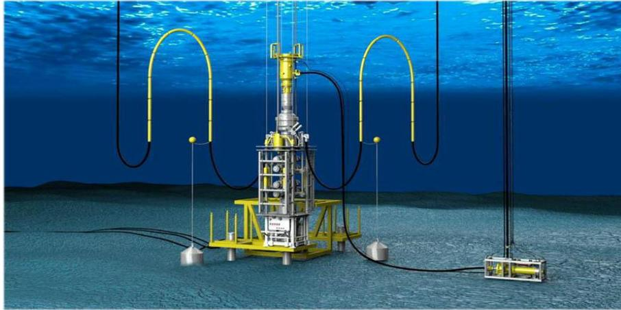
**Figure 10** ORS Riserless Drilling arrangement Figure is taken from ORS.
