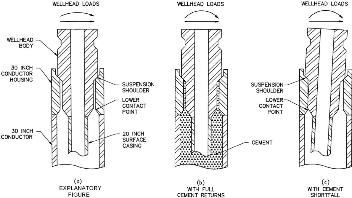
**Figure 9** Effect of cement shortfall around wellhead. Figure is taken from [18].
