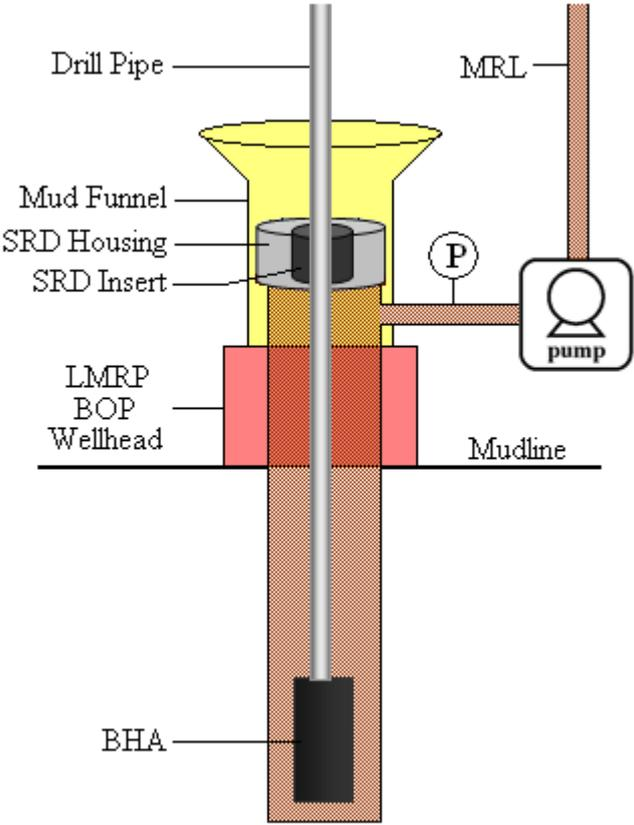
**Figure 51** A possible configuration of the combination of RD and MPD in the future.
