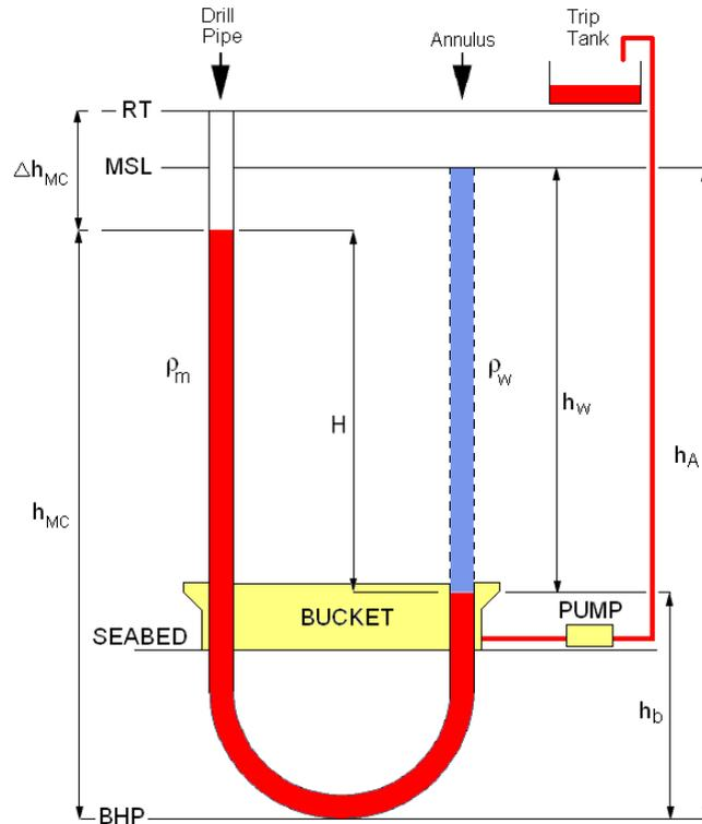
Figure 31 Illustration of the U-tube effect
