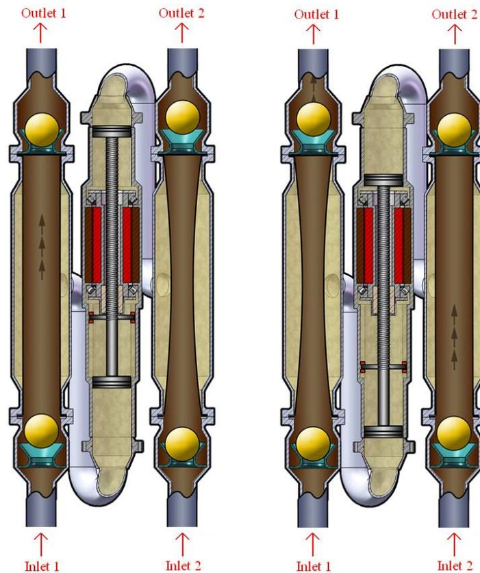
**Figure 50** PG-MAPS hose diaphragm pump configuration for one double-acting actuator. Figure is taken from [34].
