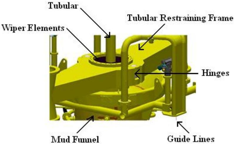
**Figure 12** *The Universal Wiper Element located on top of the Mud Funnel. Figure is taken from ORS.*
