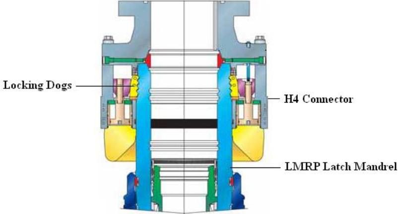
**Figure 16** VetcoGray H-4 connector cross-sectional drawing. Figure is taken from VetcoGray [22].
