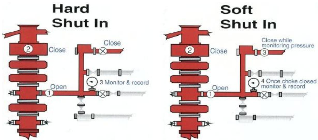
**Figure 39** Shut-in procedures of BOP and rig manifold. Figure taken from WCS [40]
