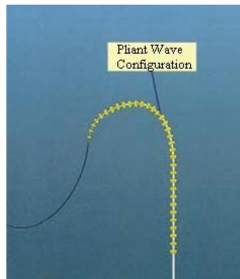
**Figure 21** Pliant Wave Configuration of k/c hoses achieved by buoyancy elements. Figure is taken from ORS.
