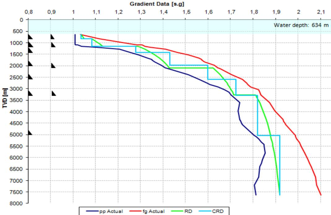
**Figure 54** Clearly showing the effect of dual gradient in terms of compatibility within the drilling window.
