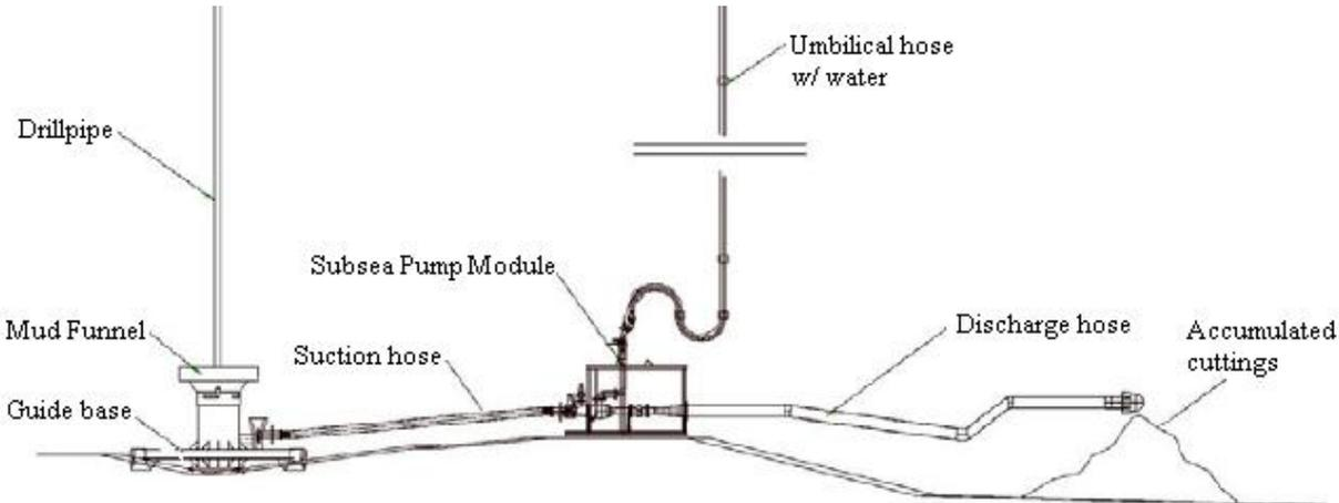
Figure 4 Cuttings Transport System schematic for IKMs injector technology. Figure is taken from IKM.
