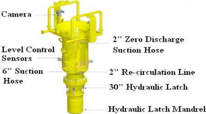
**Figure 14** ORS Mud Funnel design. Figure is taken from ORS.
