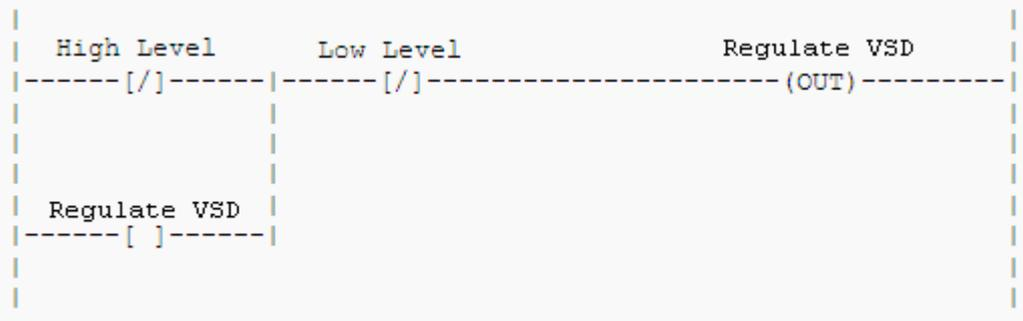
**Figure 28** Simplified circuit form for VSD control.
