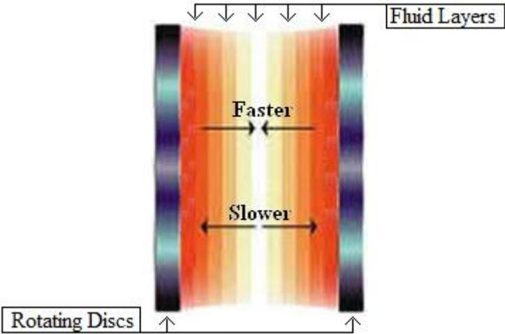
**Figure 36** Successive layers of fluid between the two rotating discs. Figure taken from [31].
