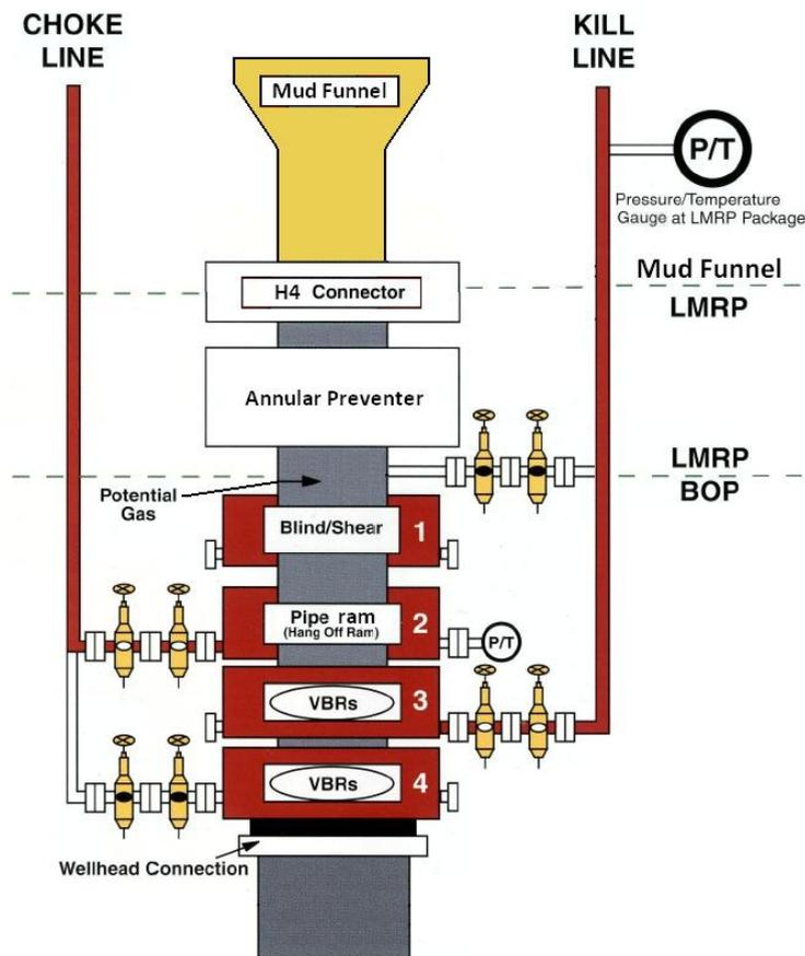
**Figure 22** The subsea arrangement of an 18 3/4" BOP stack with four rams, LMRP and Mud Funnel. Figure is taken from reference [25] and modified.
