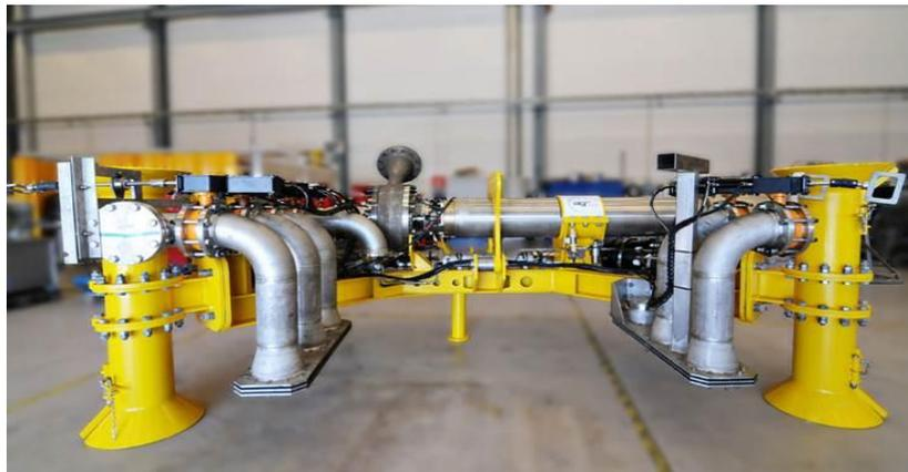
**Figure 19** AGR's Subsea Pump Module. The pump has a U-shape to allow room for the mud funnel and passage of tubular in the center. Picture is taken from AGR.
