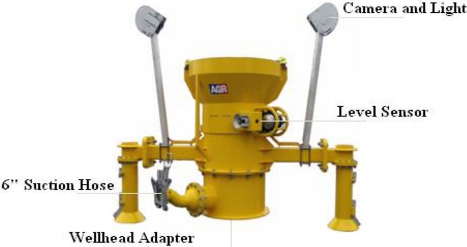
**Figure 15** AGR Mud Funnel design used for RMR<sup>®</sup> operations. Figure is taken from AGR.
