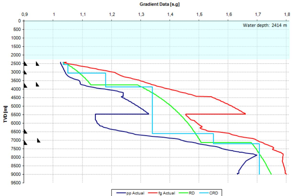
**Figure 55** Ultra deep water and the advantageous use of a dual gradient approach.
