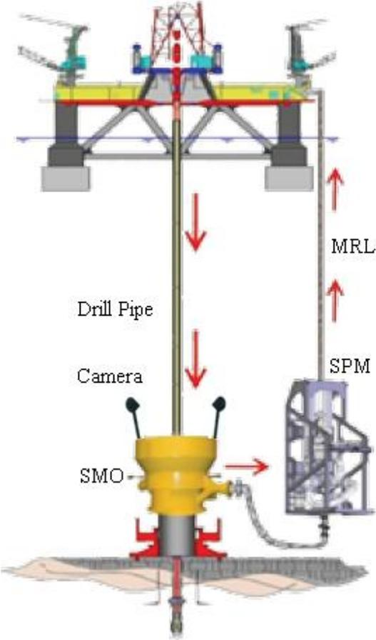
**Figure 8 RMR<sup>®</sup> Setup.** Figure is taken from AGR.
