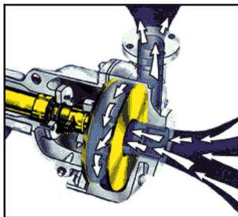
**Figure 35** Cross-sectional illustration of a disc pump. Figure taken from [32].
