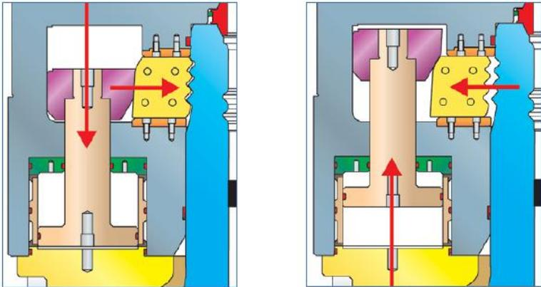
**Figure 17** Magnified preview of the hydraulic control chamber for dog ring operation Left picture is locked position, whilst right picture is released position. Figure is taken from VetcoGray [22].
