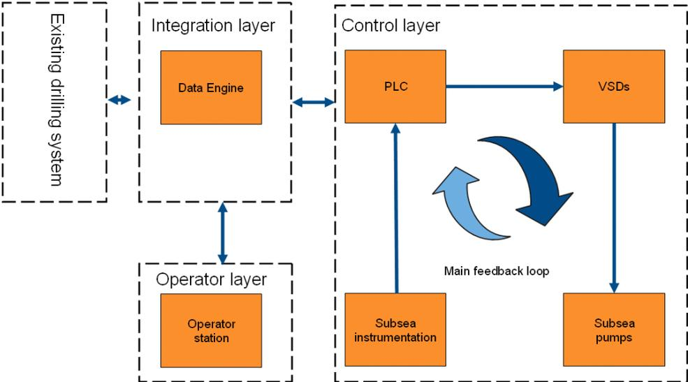
**Figure 26** Action sequence architecture for the Control System. Figure is taken from ORS.
