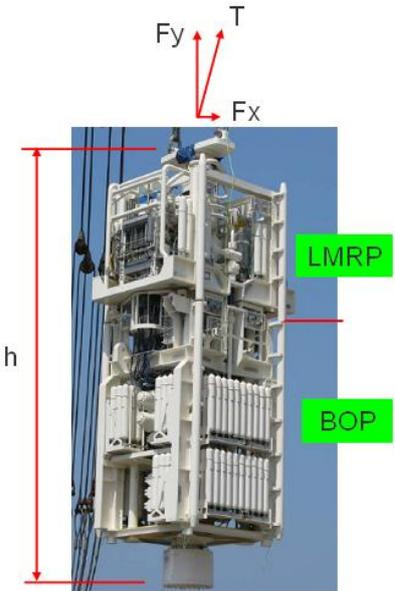
**Figure 46** LMRP/BOP stack slightly deviated to represent tensional force orientation in two dimensions. Figure is taken from [1].
