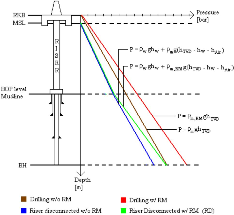
**Figure 41** Pressure plot for different scenarios during drilling and disconnect of riser. It renders the benefits of including a Riser Margin (RM) in the drilling mud.
