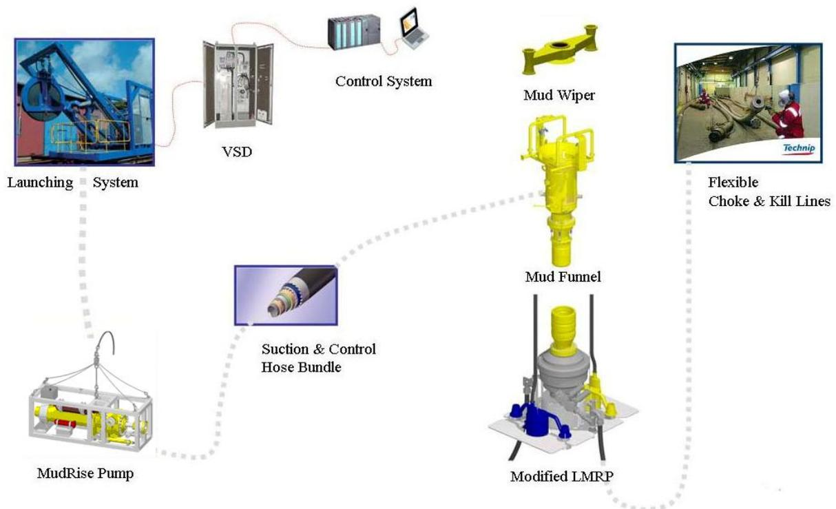
**Figure 11** ORS Riserless Drilling System Components. Figure is taken from ORS.
