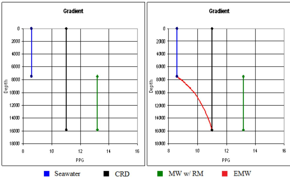
**Figure 52** Illustration of the Effective Mud Weight (EMW) while descending. Figure taken from [65].
