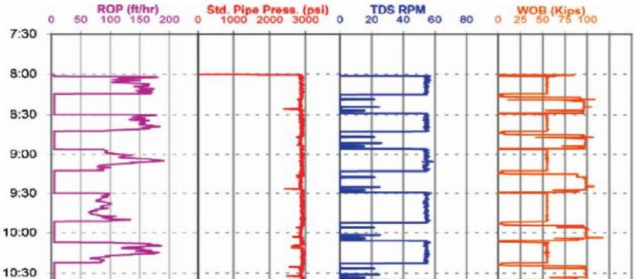
Figure 34 Data excerpt chart of CCS drilling. Figure taken from [30].
