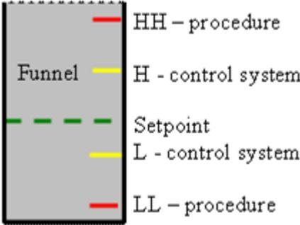
**Figure 27** Level Control System alarm boundaries. Figure is taken from ORS.
