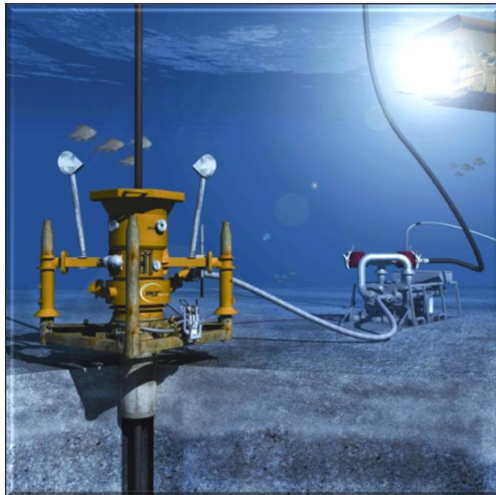
**Figure 7** Subsea arrangement of the RMR<sup>®</sup> system. Figure is taken from AGR.
