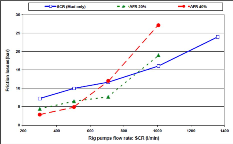
**Figure 40** Dynamic friction losses inside the choke line. Figure taken from [41]
