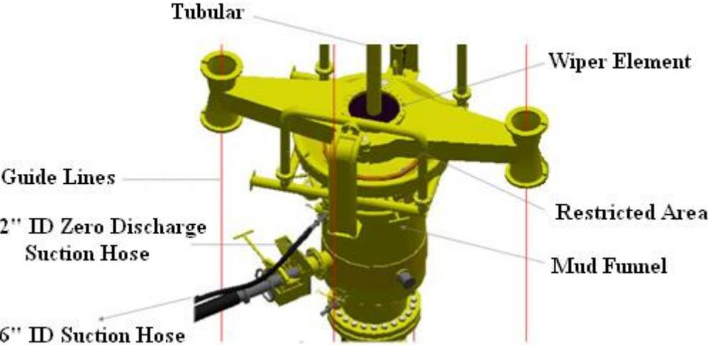
**Figure 13** Zero Discharge Arrangement on top of Mud Funnel. Figure is taken from ORS.
