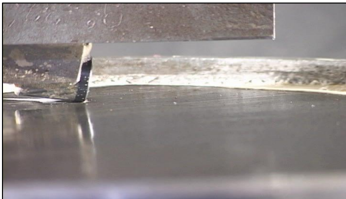
Figure 7.2: Shearing test applied to a PDC cutter on desired formation [35].
