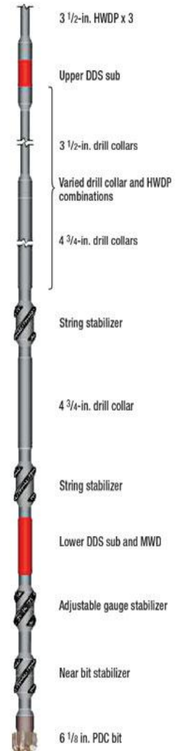
Figure 5.2: Example of a typical BHA.
