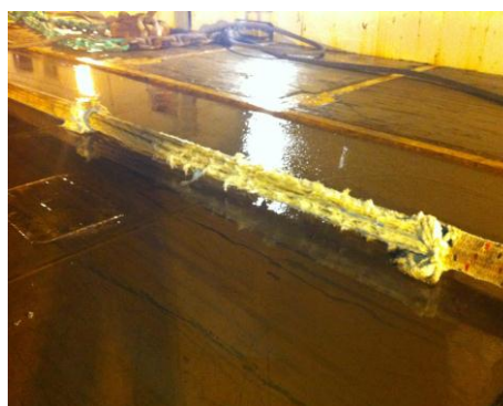
Figure 28 - Destroyed fiber rope probably harmed by a sharp edge (ref./25/).
