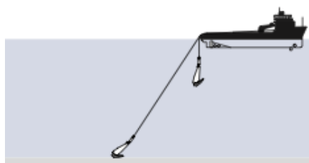
Figure 18 - Laying out anchors (ref./24/).
