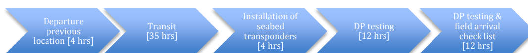
Figure 33 - Sequences of a DP rig move. Rig move distance is the same as for the towing rigs (210nm) but with a transit speed of 6 knots (ref./23/).
