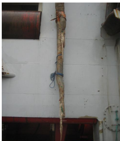
Figure 9 - Broken fiber rope (ref./25/).
