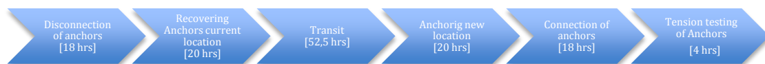
Figure 24 - Sequences of a Conventional rig move of 210nm. Assumed good weather with a transit speed of 4 knots (ref./43/).
