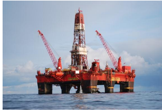
Figure 11 - West Alpha- Anchor positioned drilling rig (ref./29/).
