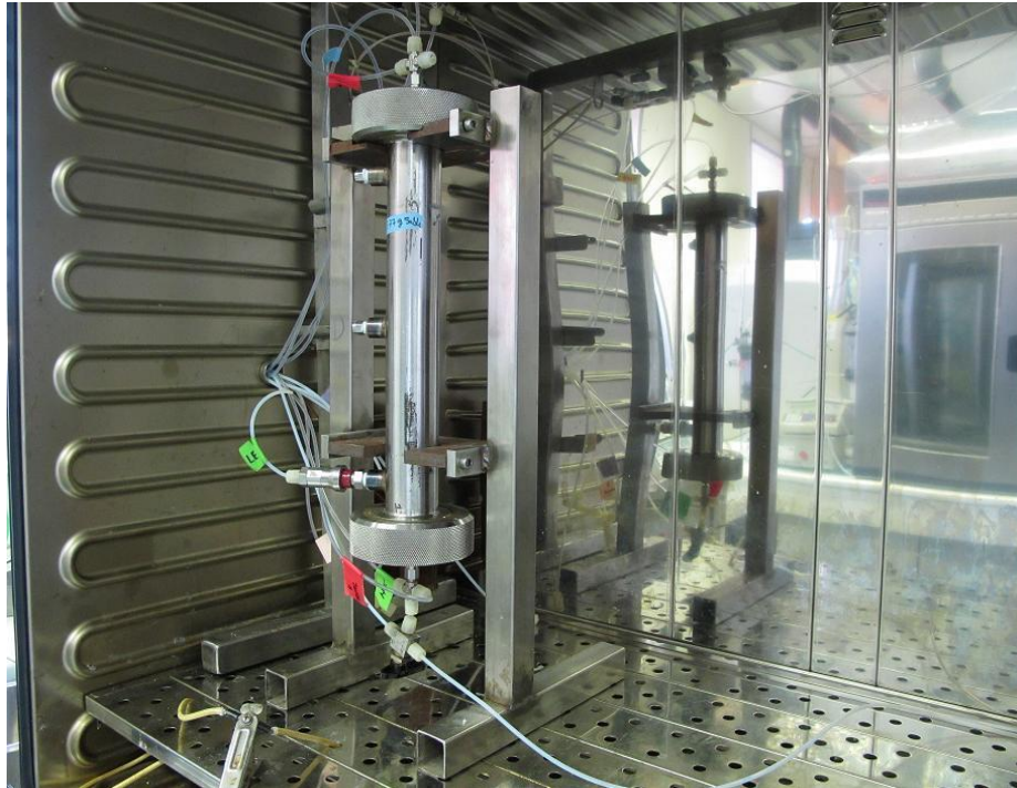
Fig. 4.9 - Sand column installed in oven.
