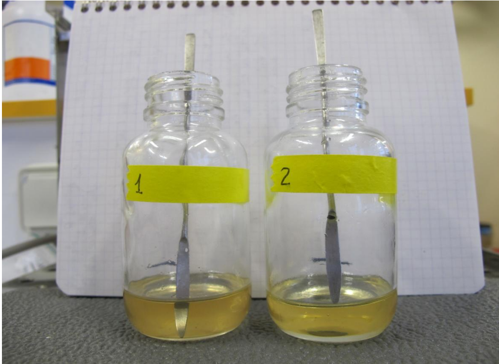
Fig. 4.22 - Samples of diluted epoxy cured at room temperature (left) and at 110 °C (right).
