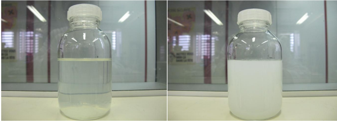
Fig. 4.13 - Effluent sample after silicate injection and after heating at 60 °C for 4 days.
