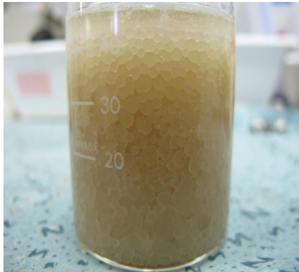
Fig. 4.17 - Water external emulsion with liquid epoxy.
