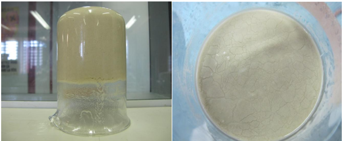
Fig. 4.4 – Fine grain sand consolidated by silicate gel.
