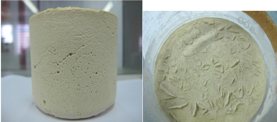
Fig. 4.5 – Fine grain sand dried out and consolidated after heating at 150 °C.
