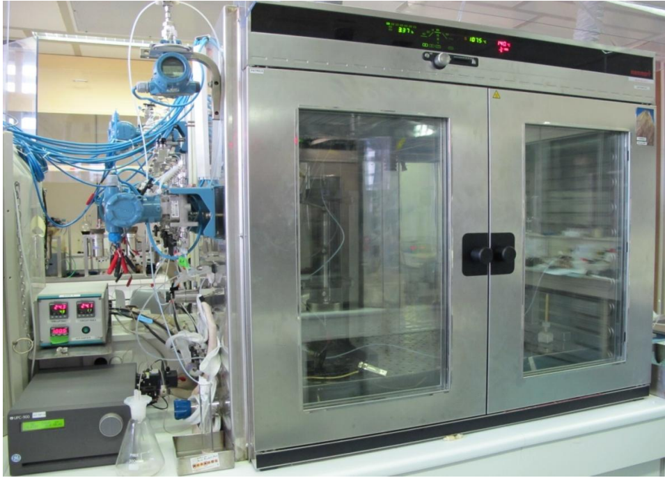
Fig. 4.15 - Sand column placed in oven for heating.
