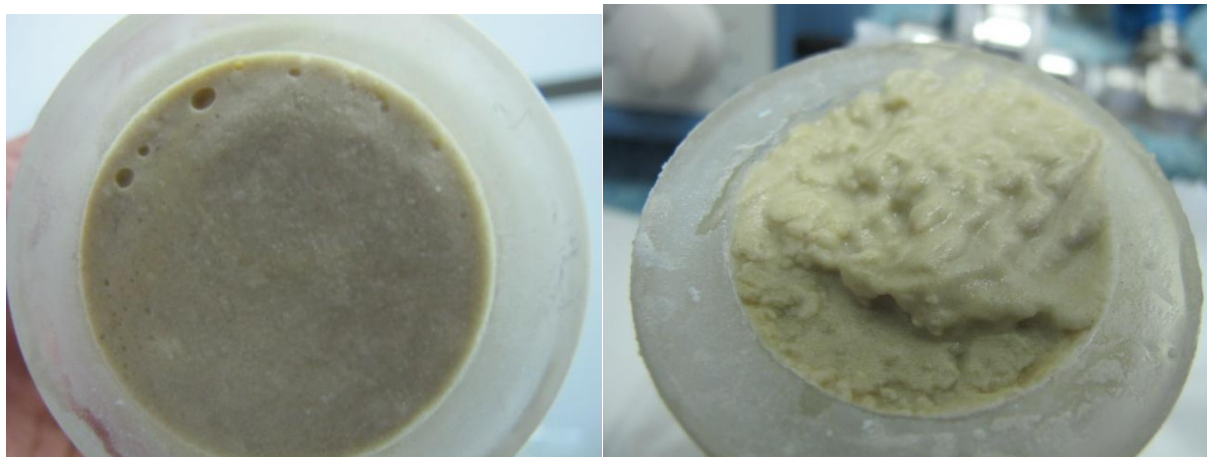
Fig. 4.8 – Gelled sand sample before and after heating by vapor.
