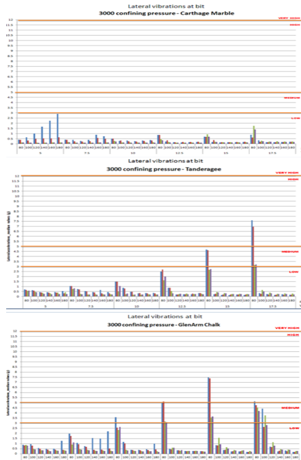
Figure 45: Lateral vibrations at bit for Carthage Marble, Tanderagee and GlenArm, from 5 to 17.5 tons, 80-180RPM. Note the increase in lateral vibrations for Tanderagee and GlenArm Carbonates compared to Carthage Marble Carbonate. (Appendix 10)
