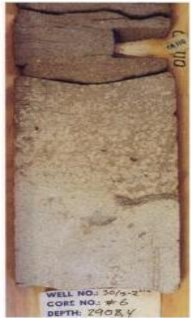
Figure 16: Patchy calcite cementation merging downwards to form an almost pervasively cemented interval. [7]
