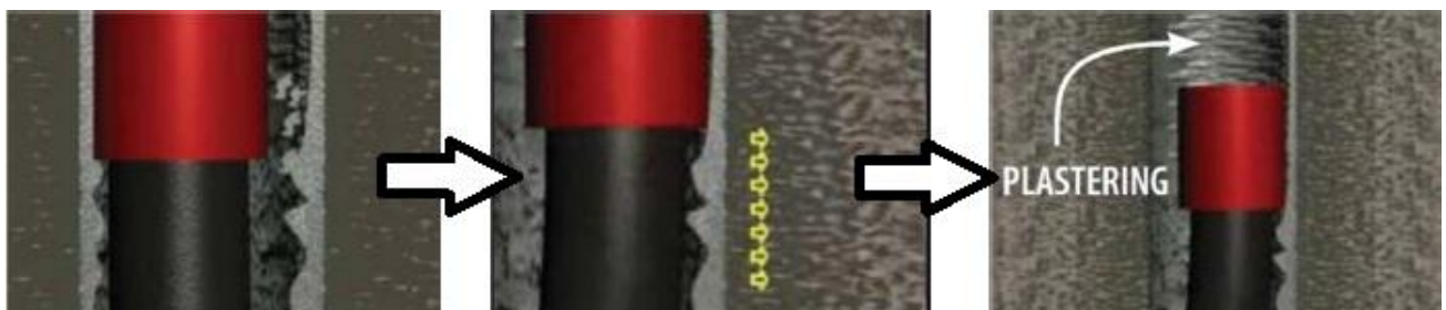
Figure 18: The plastering effect. Modified from [31].
