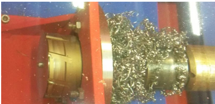
Figure 4.4 - Standard hole saw through S13Cr steel plate. The core cutaway remained stuck inside the hole saw
