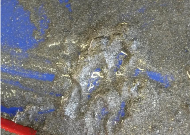
Figure 4.2 - Swarf generated from SQDS test on 13Cr. The size of the swarf can be described as small grained powder, with a mud-like texture
