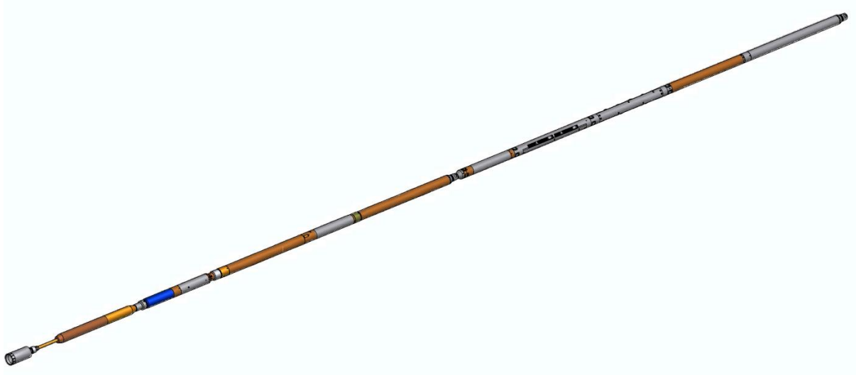
Figure 7.4 - Future toolstring design. Compared to the toolstring design presented in Chapter 2.3, the Shock Absorber is removed, and the new WOB control solution is attached directly under the DDR. The toolstring will still be in the need of a good centraliser, as close to the bit as possible
