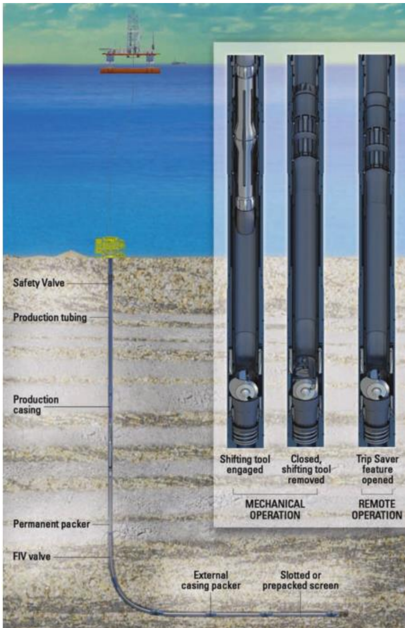
Figure 2.1 - Completion example (Schlumberger, 2009). Typically the FIV is located just above the kickoff point. Schlumberger's FIV is designed as a ball valve
