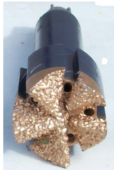
Figure 2.7 - Five bladed crushed carbide junk mill (Famco, 2013)
