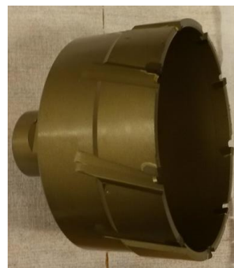
Figure 2.12 - Standard hole saw from Karnash. This hole saw was used during some of the tests. It is equipped with Sandvik tungsten carbide teeth
