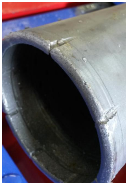
Figure 2.16 - SXDS bit. It is a diamond impregnated bit, which has been proven to work well on coiled tubing steel-milling operations
