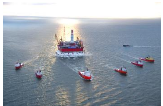
Figure 27. Platform transportation (shelf-neft.gazprom.ru)
