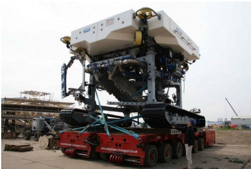
Figure 2.9: SMD Ultra Trencher - 1, worlds largest
