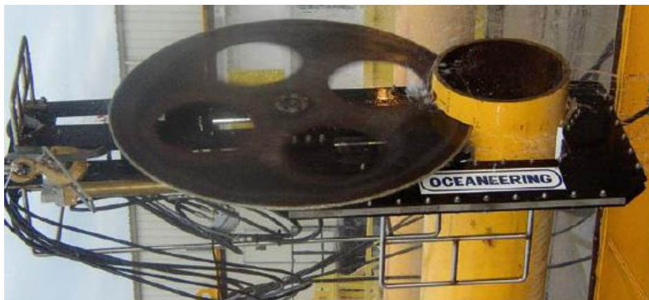
Figure 4.13: Oceanerring's ROV Deployed Chop Saw
