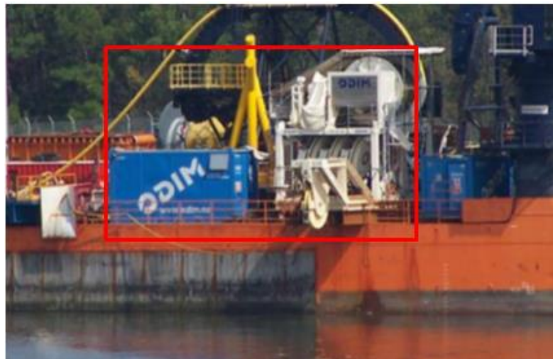
Figure 2.10: 46Te SWL, Fiber Rope Deployment System Mobilized on Toisa Perseus, REF [11], Figure.10
