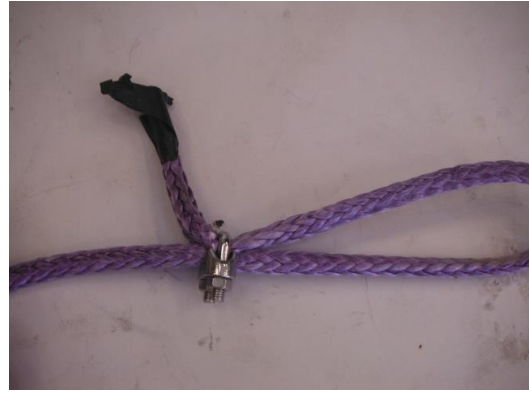
Figure 3.26: Fiber Rope Secured in a Loop
