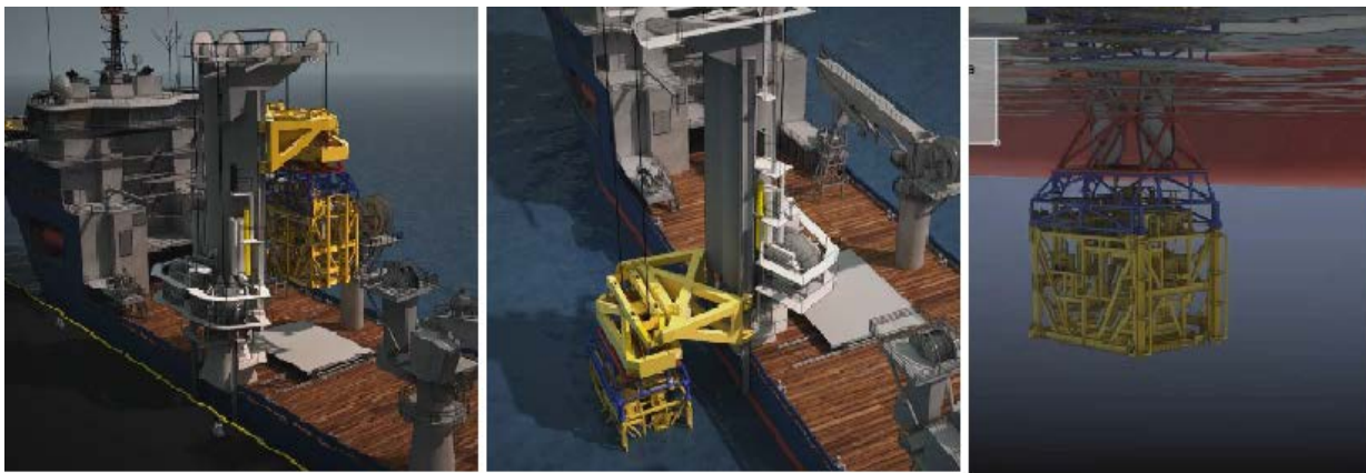
Figure 3.5: The SHS lowering a subsea module through the splash zone [29]
