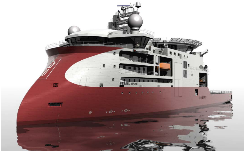
Figure 3.4: Ulsteins X-Bow ® design on an IMR vessel [26]
