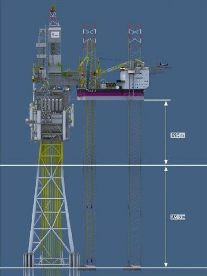
Figure 6-1 - illustration of Statoil Cat j (CJ70 design) at the Mariner field (<http://www.statoil.com/en/newsandmedia/pressroom/pages/presskitmariner.aspx>)
