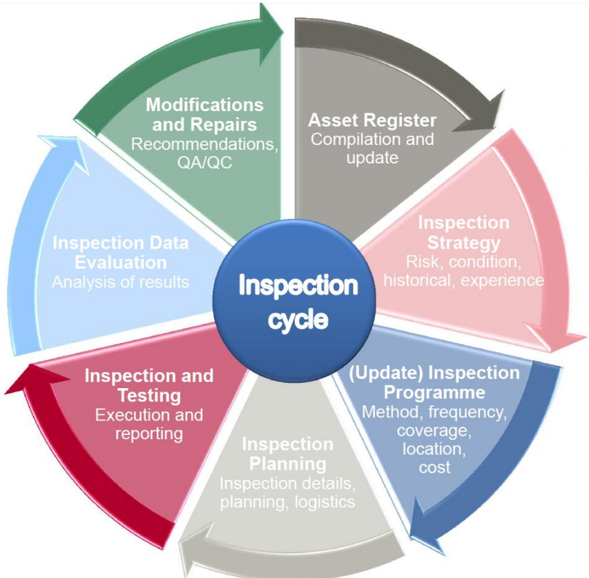
Figure 23: The inspection cycle; how all steps relate to each other (Bureau Veritas, 2014)
