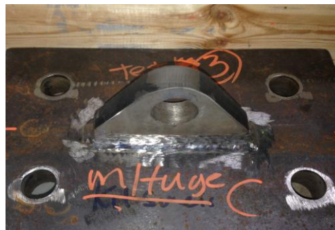
Test 3, vertical: Deformation of 3.5 mm in the pad eye hole.
