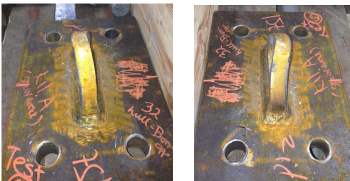
Test 6, angular: Large deformation and twisting of the ear.
