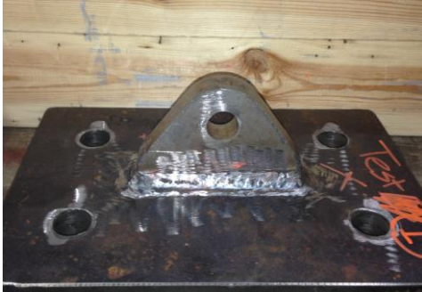
Test 1, vertical: Deformation of 0.5 mm in the pad eye hole.
