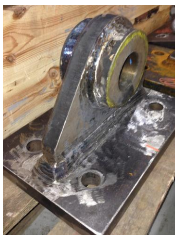
Figure 4.4: Finished test sample of the modified 12 ton pad eye.
