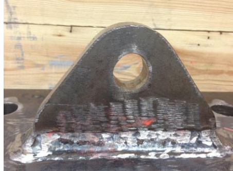
Test 1, vertical: Deformation of 0.5 mm in the pad eye hole.
