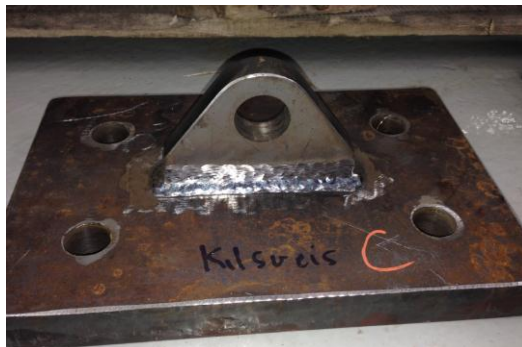
Figure 4.3: Finished test sample of a 3.25 ton pad eye.
