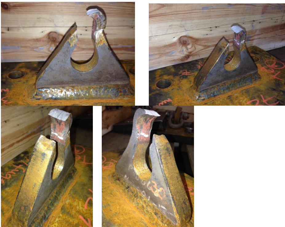
Test 9, vertical: Fractured and cracked pad eye.
