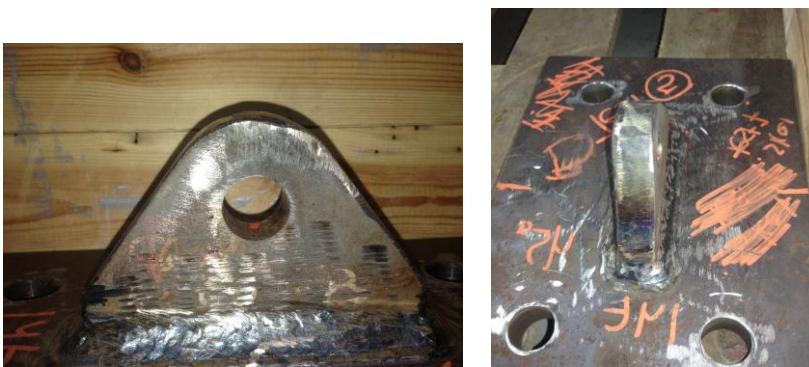
Test 5, angular: Deformation and twisting of the Pad eye.
