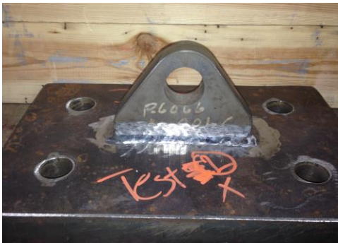
Test 2, vertical: Deformation of 1.5 mm in the pad eye hole.
