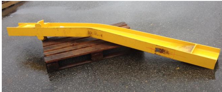
The IPE beam after the testing twisted and deformed.
