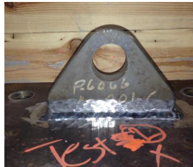
Test 2, vertical: Deformation of 1.5 mm in the pad eye hole.
