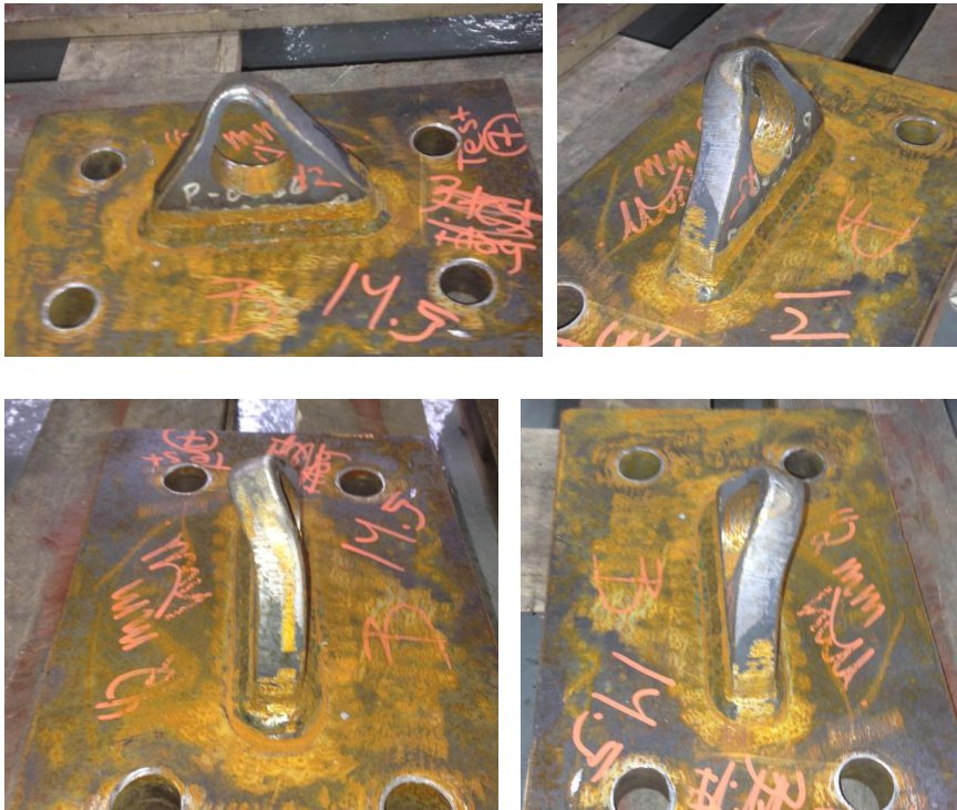
Test 7, angular: Very large deformation and significant twisting of the ear.
