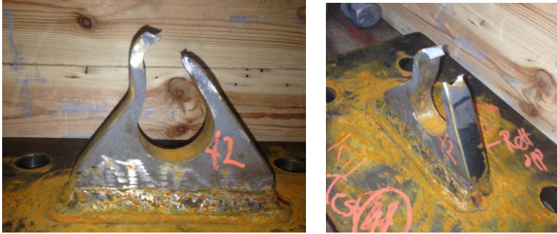
Test 4, vertical: Fractured pad eye.
