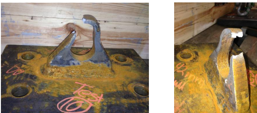
Test 10, vertical: Fractured and deformed pad eye.
