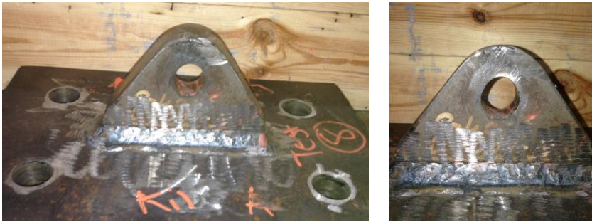
Test 8, vertical: Deformation of 1.5 mm in the pad eye hole.
