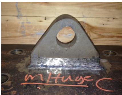
Test 3, vertical: Deformation of 3.5 mm in the pad eye hole.
