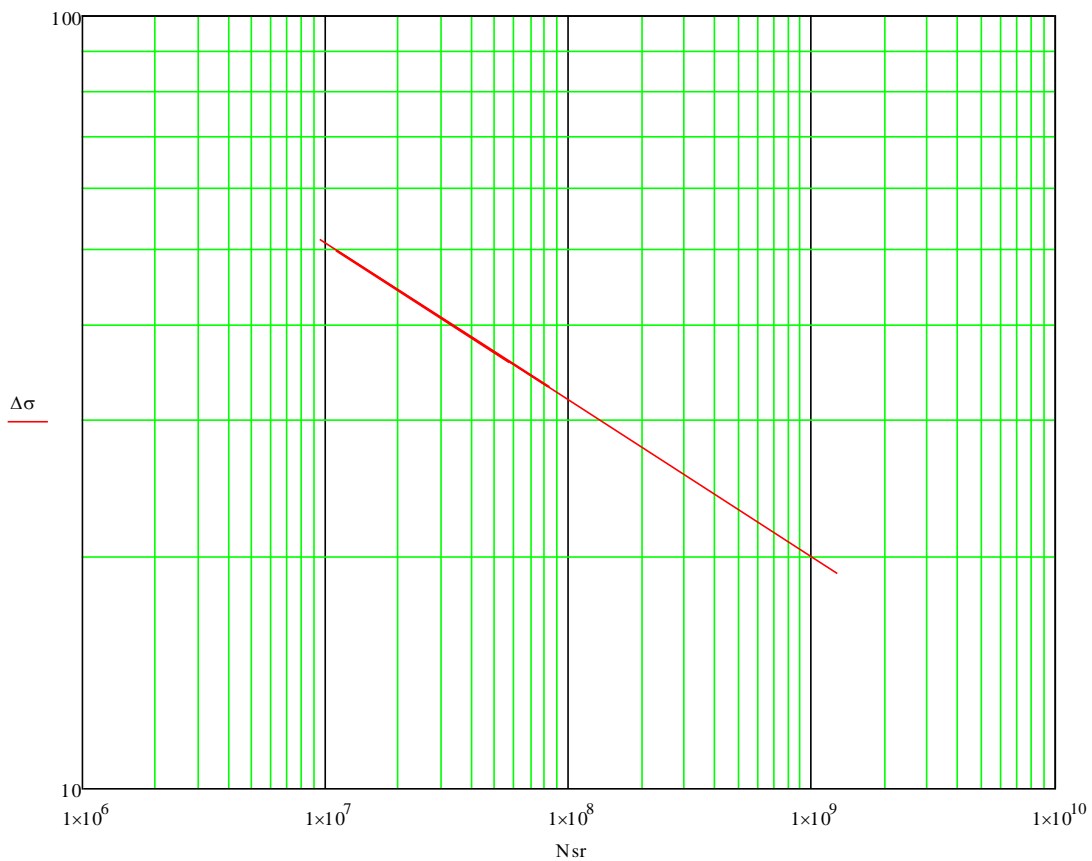
Figure 49 S-N curve between years 1951-1970 by using Mathcad
