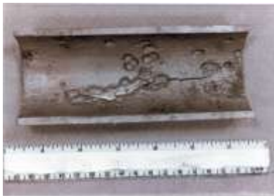
Figure 5 Example of pitting corrosion in a pipe [21]
