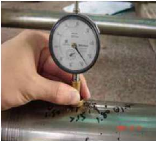
Figure 9 Measuring depth of pitting deep (pit gauge) [22]
