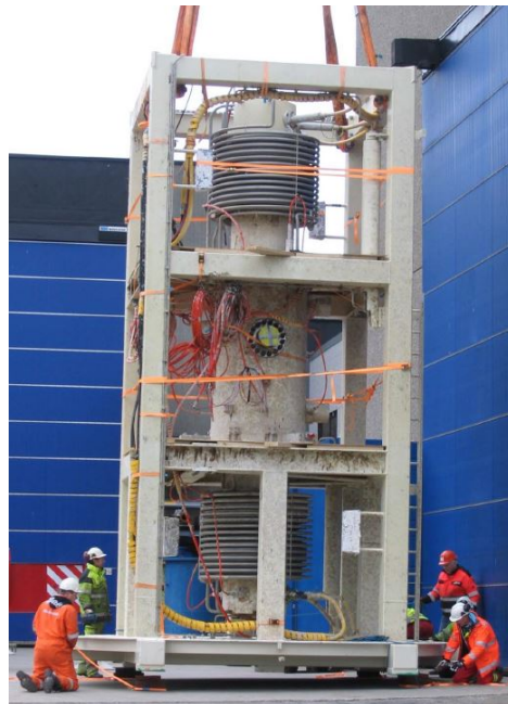
Figure 3.14 Wet gas compressor for Gullfaks (Wadel-Andersen, no date)
