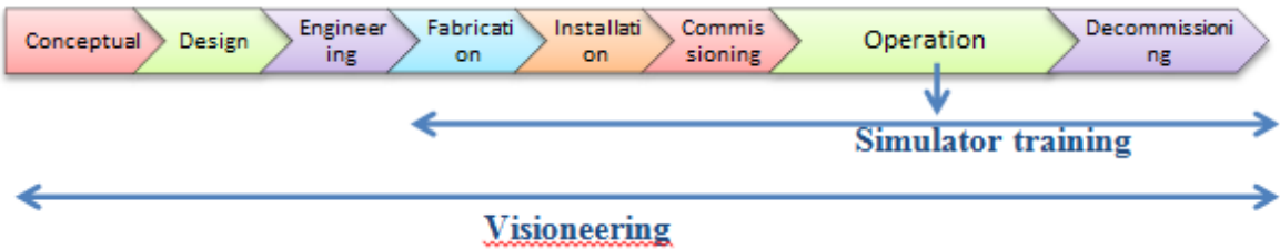
Figure 6.5 Rig Project Lifecycle Management.
