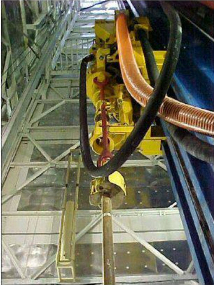
Figure 4 - The pipe handling machine [24]
