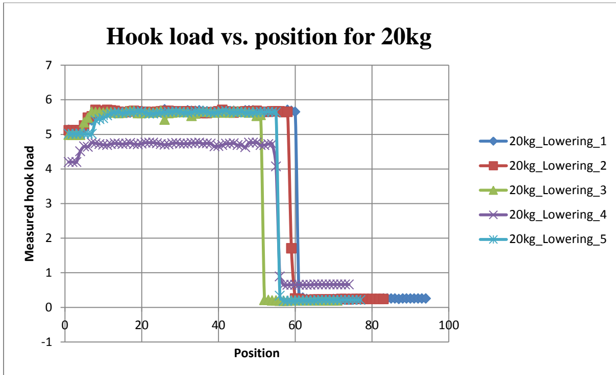
Figure 36 - Plot of hook load against position for five different experiments for 20kg
