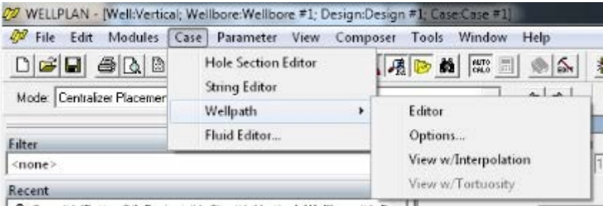
Figure 5.6: The data needed for calculations must be entered under the "case" menu.
