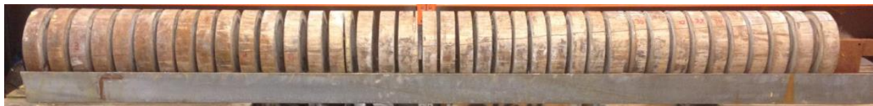
Figure 55: The casing cut into 7.5 cm pieces (Hydrawell, 2014f)
