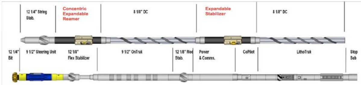
Figure 35: BHA 2, expandable stabilizer above the reamer [37]
