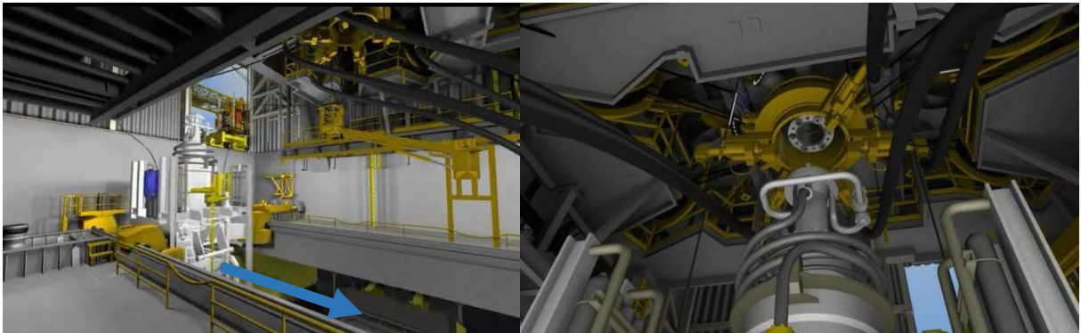
Figure 18 BOP skidded to center of moon pool (l.s) and first riser joint coming through from drill floor (r.s) [46]
