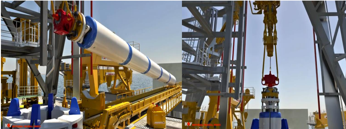
Figure 10 Riser joint picked up from the catwalk machine (l.s) and ran through the spider (r.s) [33]
