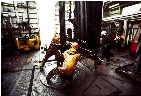
Figure 4 Drilling crew breaking out a connection using manual rig tongs [19, 20]
