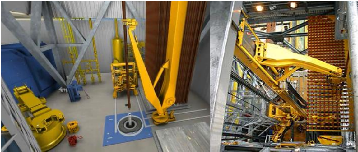
Figure 6 The X-Y Hydraracker lifting pipe to the well center (l.s) and seen from above getting pipe from the fingerboard (r.s) [22, 23]
