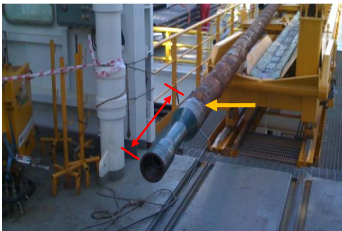
Figure 46 Drill collar with lifting sub mounted on
