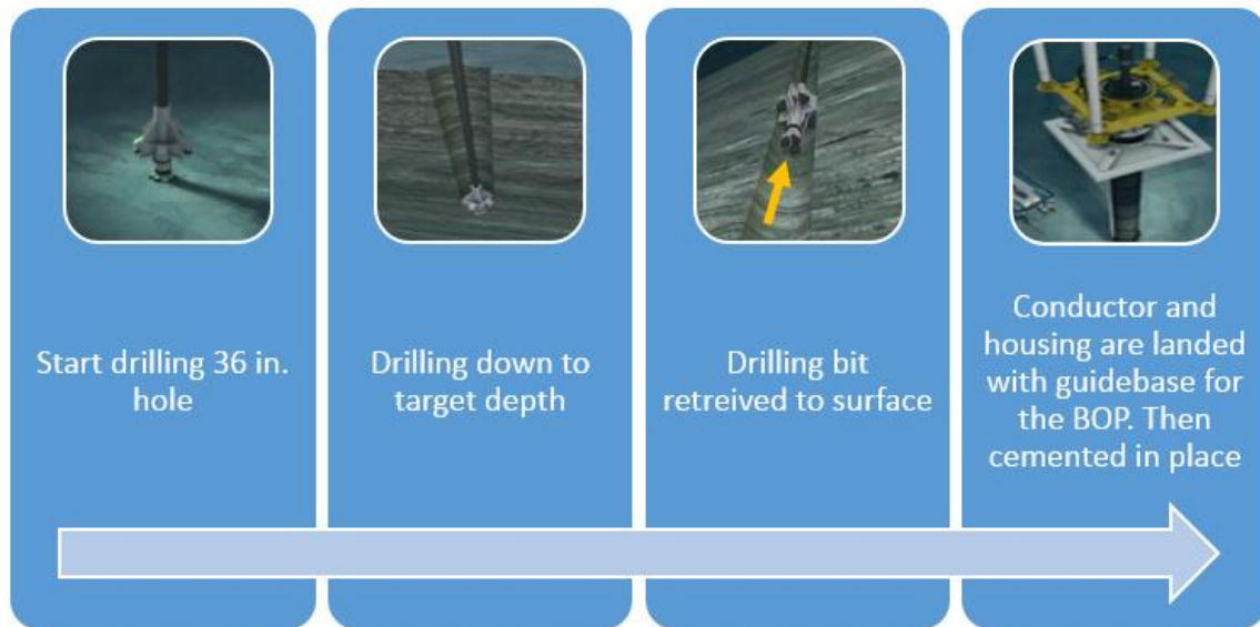
Figure 13 Drilling 36 in. hole and run 30 in. conductor with guide base [40]
