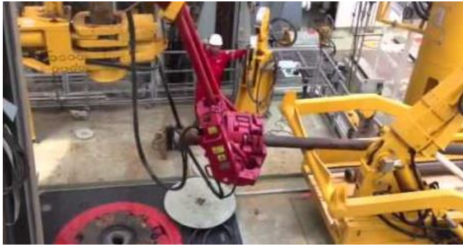
Figure 47 The elevator (red module) is ready to lift the pipe out of the catwalk
