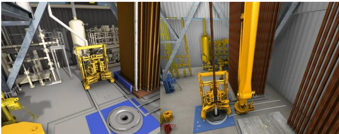
Figure 3 Iron roughneck on the drill floor in parked position (l.s) and while making up a connection (r.s) [17]
