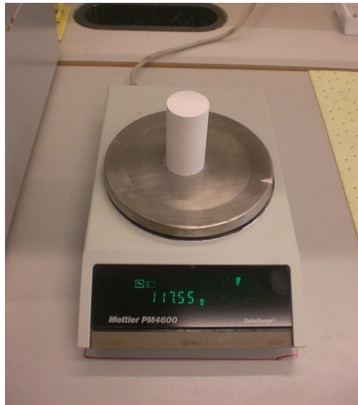
Figure 3.4 – Measuring weight of the core by weighting-machine.
