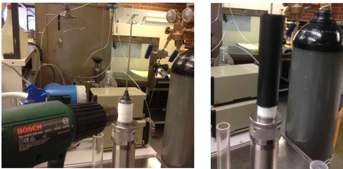
Figure 21 – Heating of plastic cover and putting rubber cover
