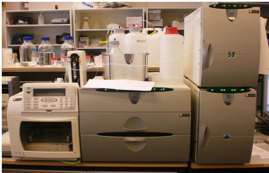
Figure 25 - Dionex ICS-3000 chromatograph
