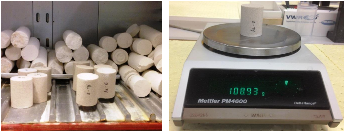
Figure 17 – Oven with cores and weighing of core
