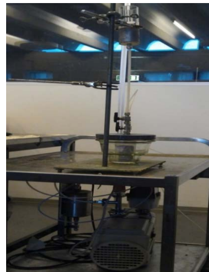
Figure 11.19. Water Saturation Setup
