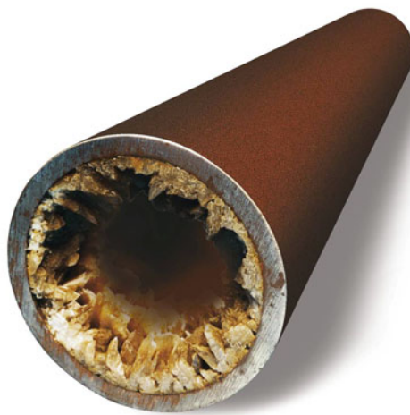
Figure 2.1 Scale deposit in a pipe [4]
