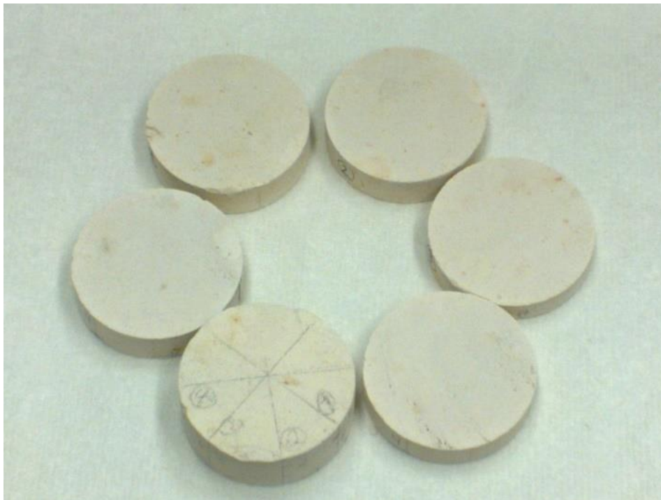
Figure 3-12: The KA9-L core after cutting and ready for pycnometer measurements
