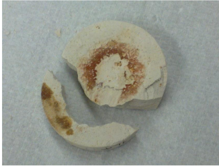
Figure 5-1: Broken KA9-L core piece from the inlet side.
