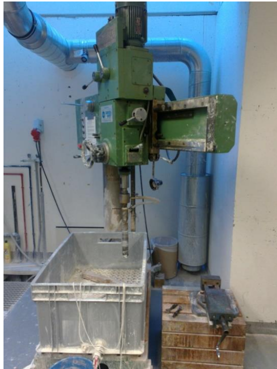
Figure 3-1: The drilling machine used for drilling the cores out from the Kansas chalk block.
