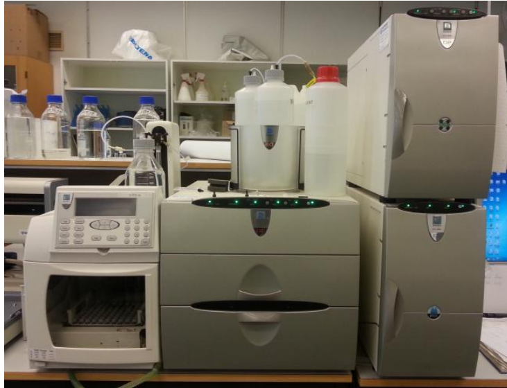
Figure 3-14: The Dionex ICS-3000 Ion Chromatography
