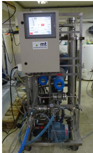
Figure 5-5 NANO-BW-4040 Membrane Installation
