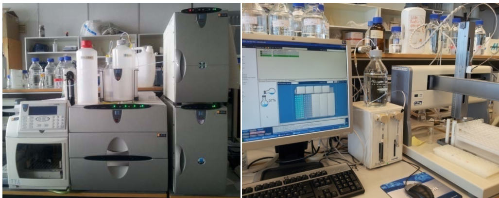
Figure 5-8 Dionex ICS – 3000 Instrument (left) and Dilution Machine (right)
