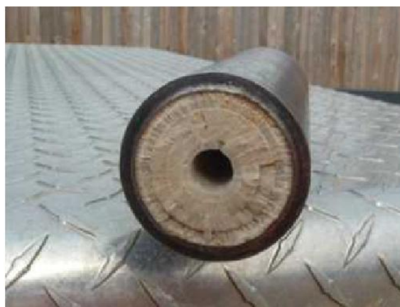
Figure 2-4 \text{BaSO}_4 Scale in Haynesville Shale Flow Line after One Month (Meehan, 2010)
