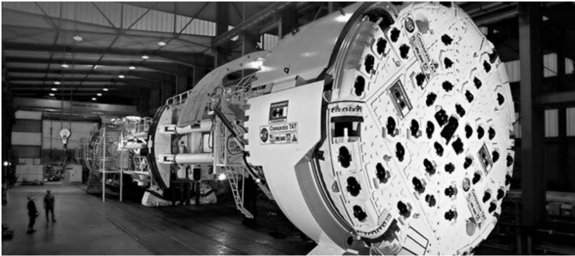
Figure 3-10 Tunnel boring machine (TBM)
