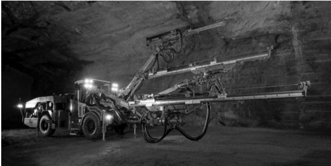
Figure 3-8 Example of a three arm (three-boom) hydraulic drill rig
