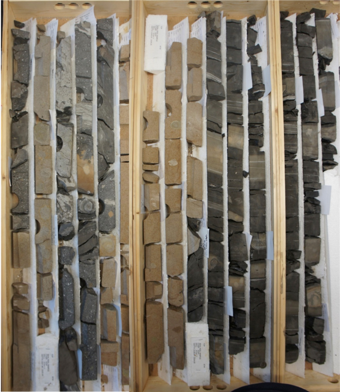
Appendix 2, complete image of the cored interval of the Knurr Formation in well 7019/1-1. Top of core (2220.0m TVD) is top left, bottom of the core (2234.3m TVD) is bottom right. Parts of the core is missing due to seal peel or sampling.
