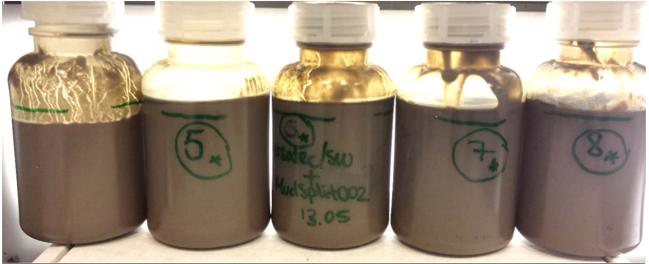
Figure 4.15 Versatec OBM (50/50) + MudSplit002 added at following concentrations (left to right) Blank, 0.50 (# 5*), 2.00 (# 6*), 3.00 (# 7*) and 5.00 vol/vol % (# 8*).
