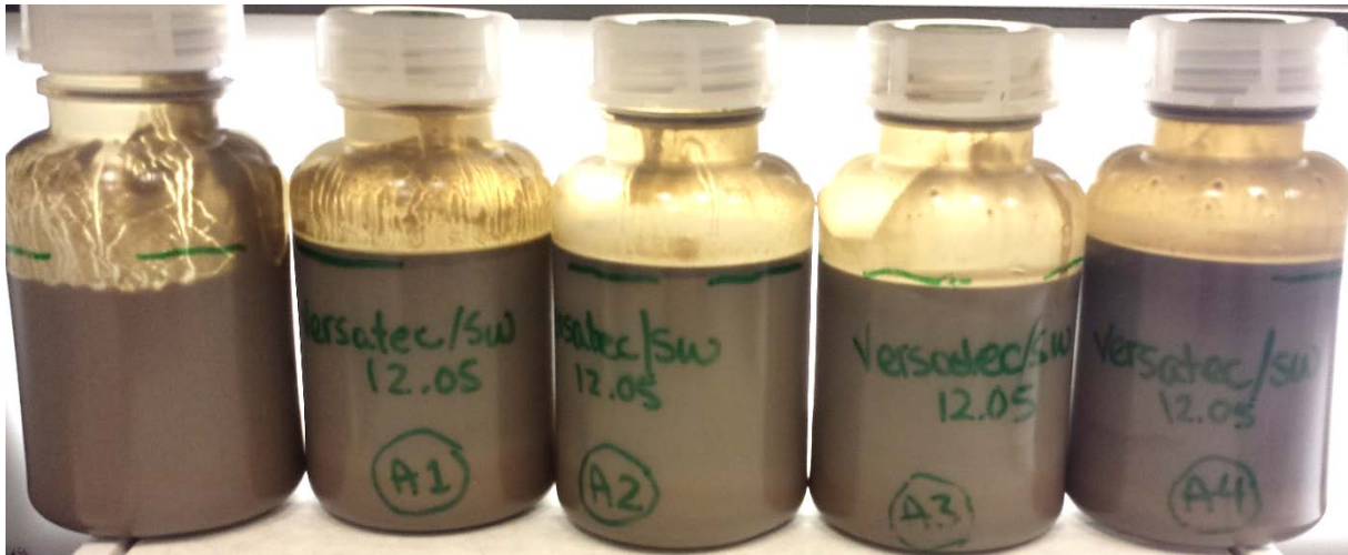
Figure 4.17 Versatec OBM (50/50) + MudSplit004 added at following concentrations (left to right): Blank, 0.25 (# A1), 0.50 (# A2), 1.00 (# A3) and 2.00 vol/vol % (# A4).
