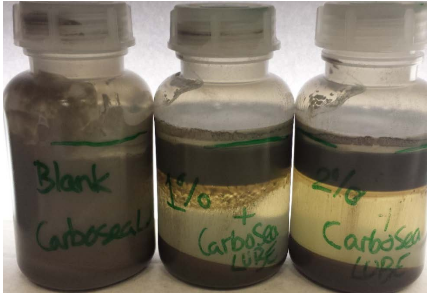
Figure 4.20 Carbosea LC-LUBE Fine Premix OBM (50/50) + MudSplit005 added at following concentrations (left to right) Blank, 1.00 % and 2.00 vol/vol %.
