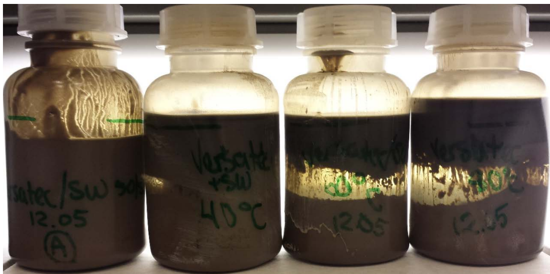
Figure 4.21 Bottles with following temperature adjustments (left to right) 20°C (# A), 40°C, 60 °C and 80 °C.
