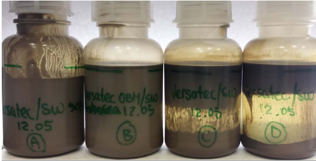
Figure 4.18 Versatec OBM (50/50) + MudSplit005 added at following concentrations (left to right): Blank (# A), 0.50 (# B), 1.00 (# C) and 2.00 vol/vol % (# D).
