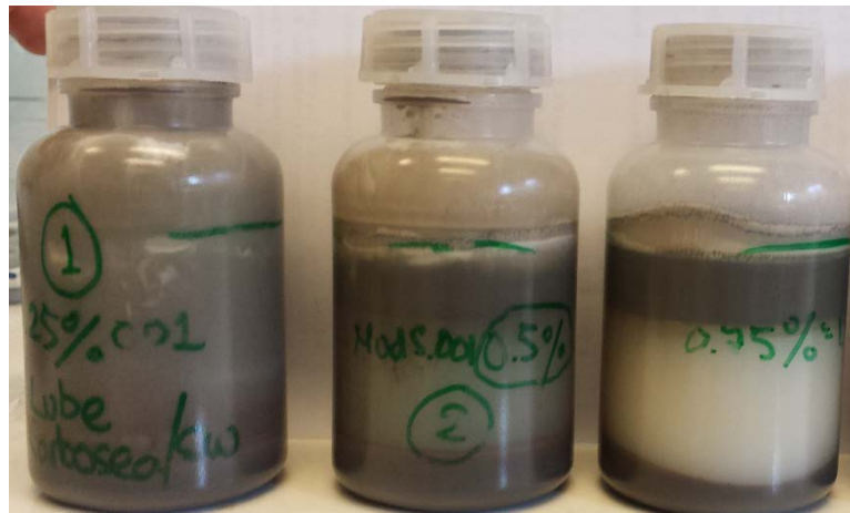
Figure 4.19 Carbosea LC-LUBE Fine Premix OBM (50/50) + Mudsplit001 added at following concentrations (left to right) 0.25 (# 1), 0.50 (# 2), 0.75 vol/vol % (# no label).
