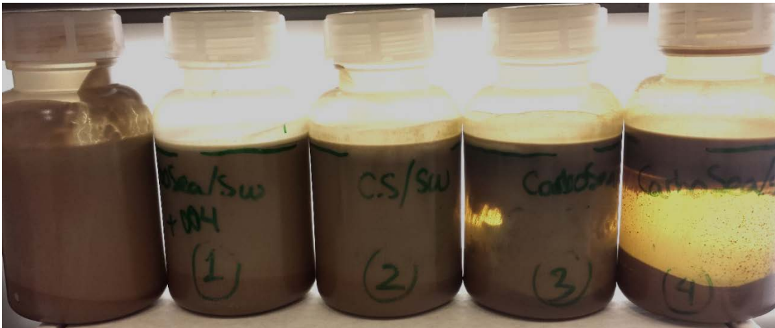
Figure 4.13 Carbosea OBM (50/50) + MudSplit005 added at following concentrations (left to right): Blank, 0.25 (# 1), 0.50 (# 2), 1.00 (# 3) and 2.00 vol/vol % (# 4).
