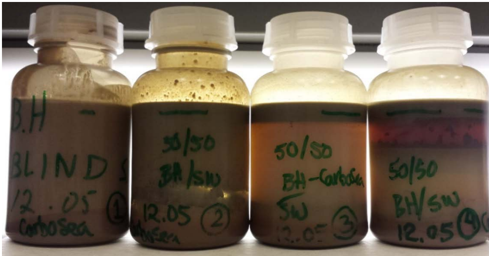
Figure 4.10 Carbosea OBM (50/50) + MudSplit001 added at following concentrations (left to right) Blank (# 1), 0.50 (# 2), 2.00 (# 3) and 5.00 vol/vol % (# 4).
