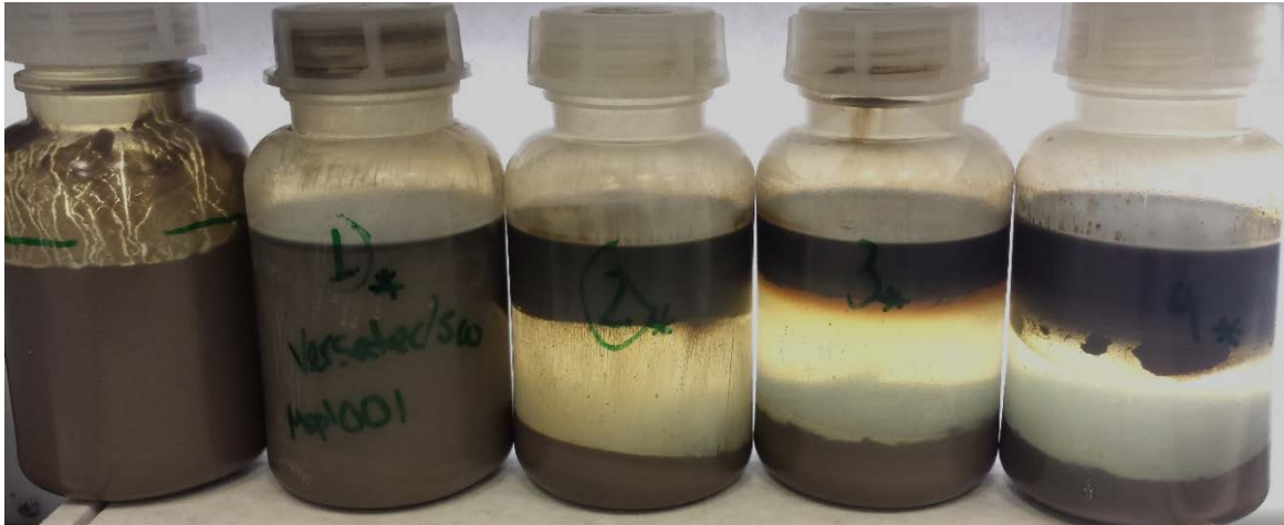
Figure 4.14 Versatec OBM (50/50) + MudSplit001 added at following concentrations (left to right) Blank, 0.25 (# 1 x ), 0.50 (# 2 x ), 2.00 (# 3 x ) and 5.00 vol/vol % (# 4 x ).
