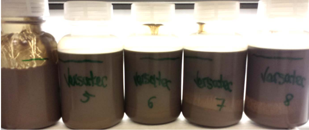
Figure 4.16 Versatec OBM (50/50) + MudSplit003 added at following concentrations (left to right) Blank, 0.25 (# 5), 0.50 (# 6), 2.00 (# 7) and 5.00 vol/vol % (# 8).
