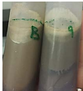
Figure 4.7 Centrifuge bottles directly after centrifuging. Blank sample of Carbosea OBM (# B) and with 2.00 % MudSplit005 (# 9).
