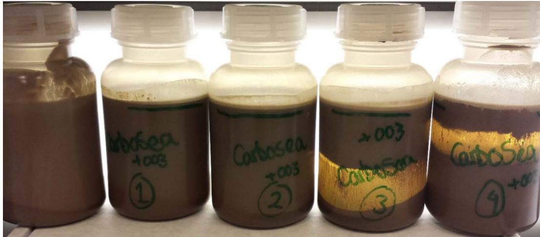
Figure 4.12 Carbosea OBM (50/50) + MudSplit003 added at following concentrations (left to right) Blank, 0.25 (# 1), 0.50 (# 2), 2.00 (# 3) and 5.00 vol/vol % (# 4).
