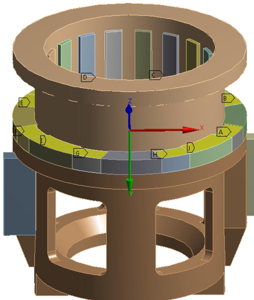
Figure 95: SGB and gear housing displacement supports
