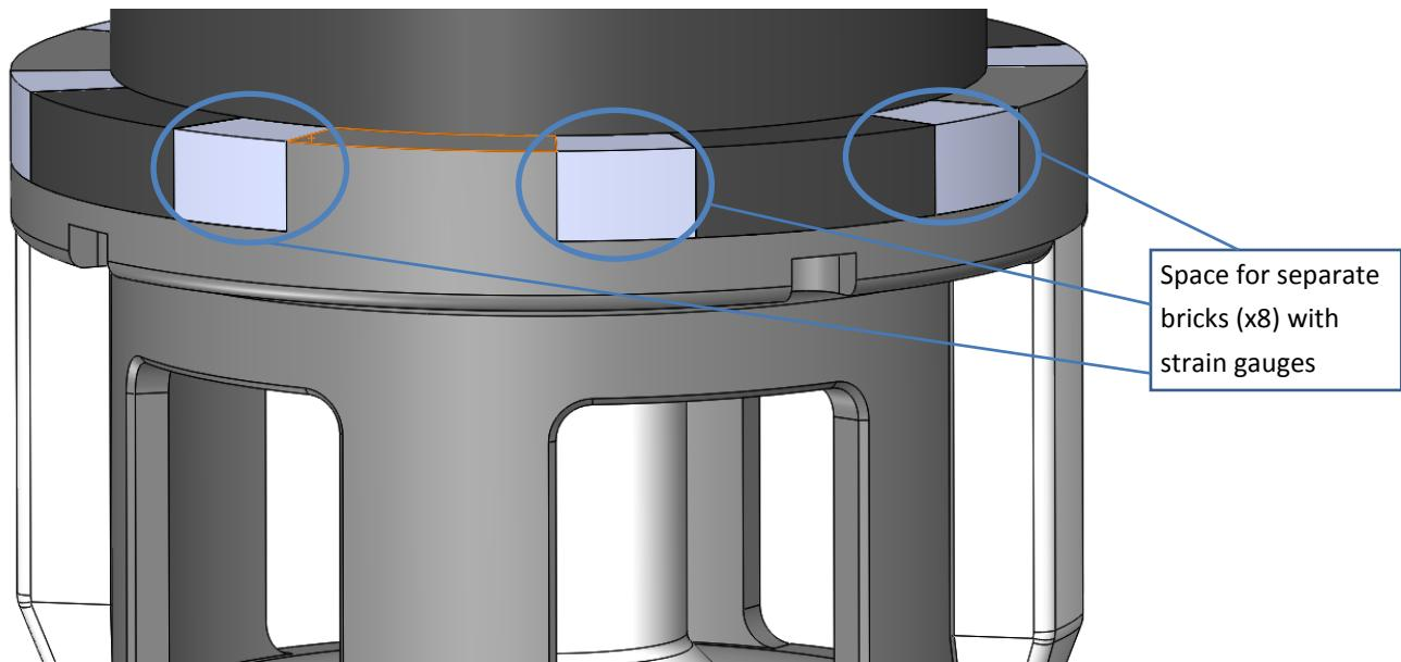
Figure 38: Measuring between gear housing and tool guide
