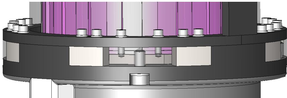
Figure 44: Transducer assy, gear housing and tool nose guide assembled
