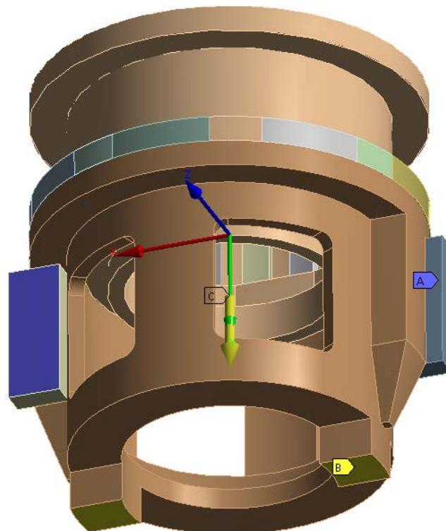
Figure 93: Reaction plates fixed support and tool guide displacement support
