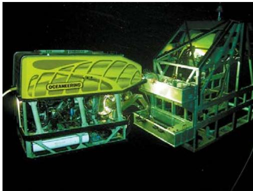
Picture 2: ROV behind a TMS (cage type) [7]
