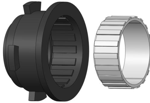
Figure 53: Ring gear and gear housing exploded view
