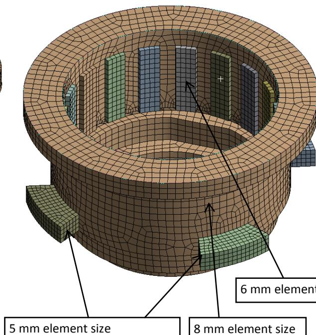
Figure 102: Gear housing multi-body part mesh
