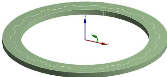
The simplified gear housing and the ring gear with the cylindrical coordinate system is shown to the left. The moment is acting counter clockwise.
