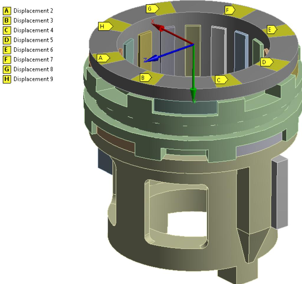
Figure 70: Gear housing displacement supports
