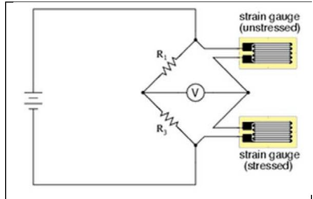
Figure 22: Quarter bridge with temperature compensation [11]
