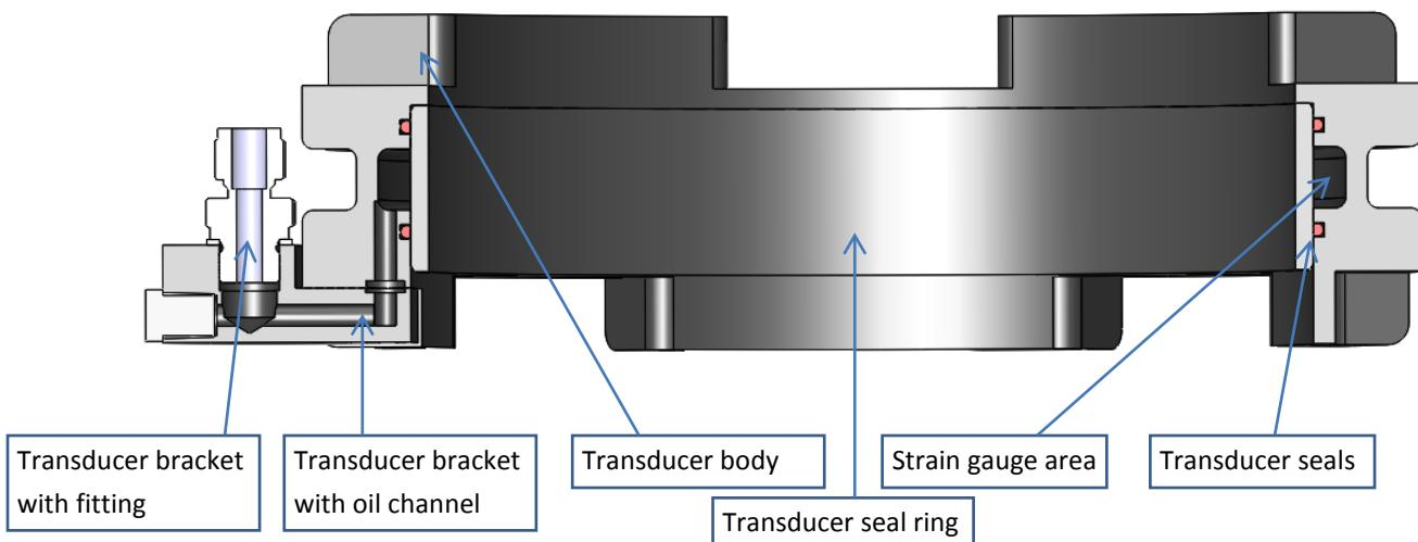
Figure 19: Torque transducer section cut
