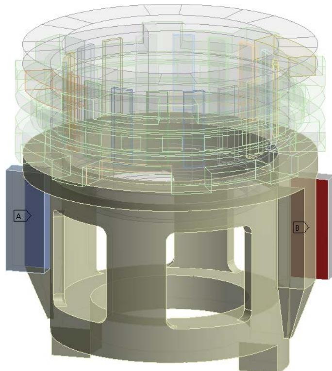
Figure 79: Tool guide and reaction plate contacts
