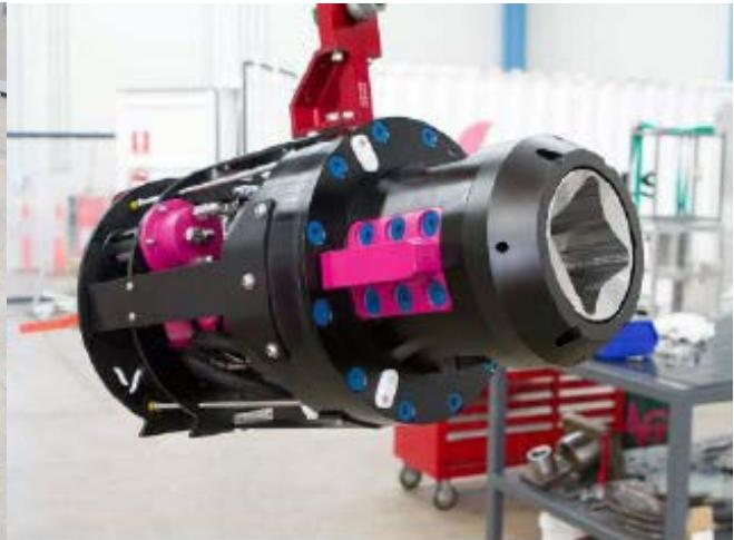
Picture 5: Velocious torque tool lifted
