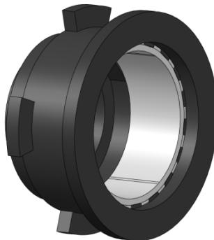
Figure 52: Ring gear and gear housing
