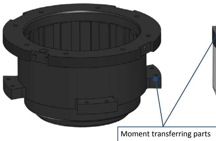
Figure 40: Gear housing
