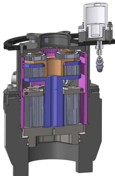
Figure 15: OAS TT Gearbox design
