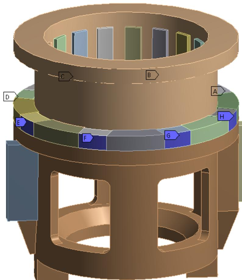
Figure 94: Cylindrical support on SGBs
