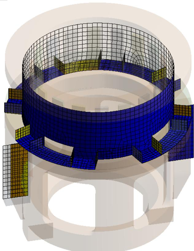
Figure 103: Final contacts for new concept analysis
