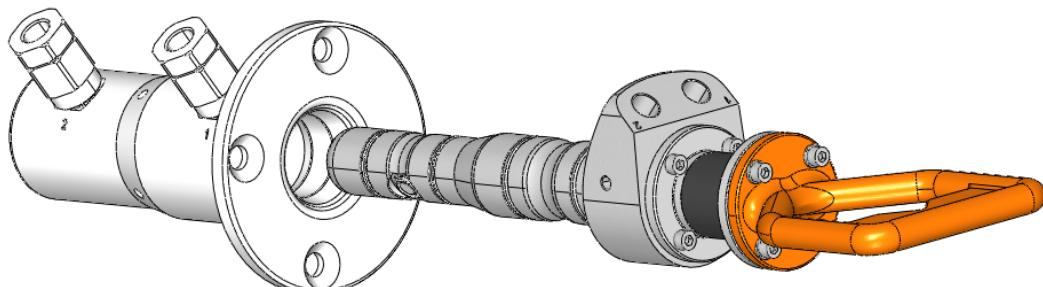
**Figure 7: Receptacle and hot stab**
