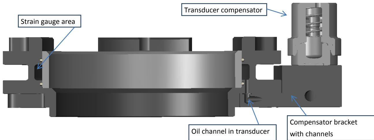
Figure 12: Section cut of torque transducer
