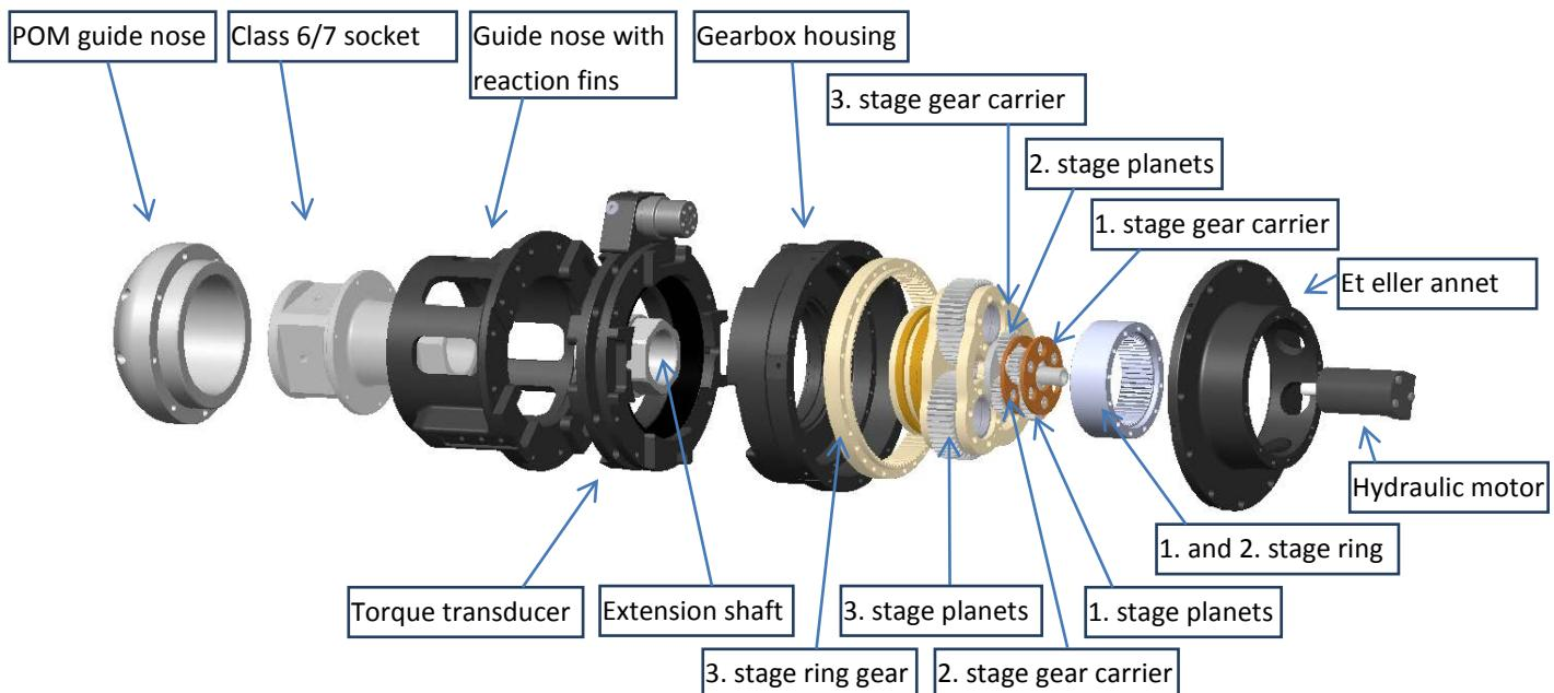
Figure 9: SAE TT exploded view of model
