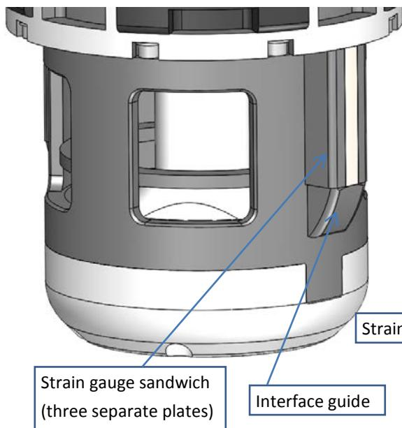
Figure 36: Strain gauges in reaction fins
