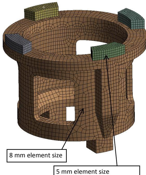
Figure 101: Tool guide multi-body part mesh
