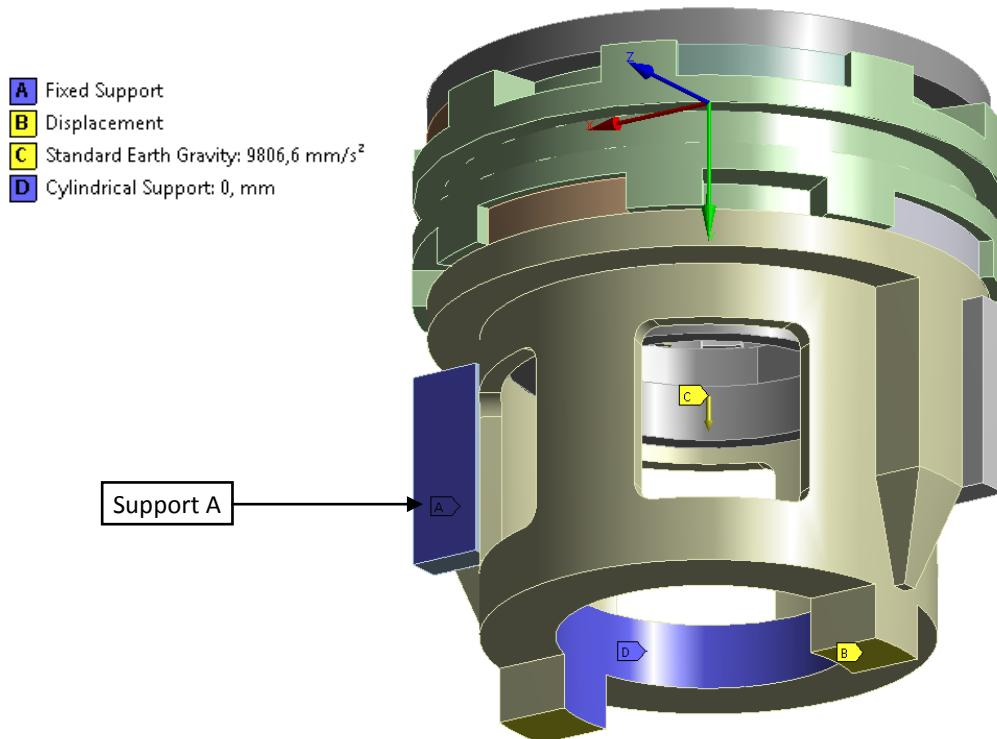
Figure 69: Tool guide and reaction plates supports
