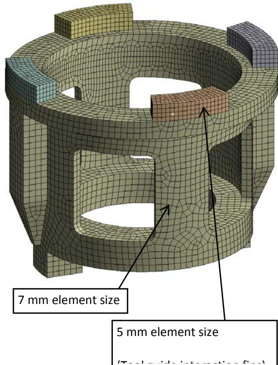
Figure 83: Tool guide multi-body part mesh
