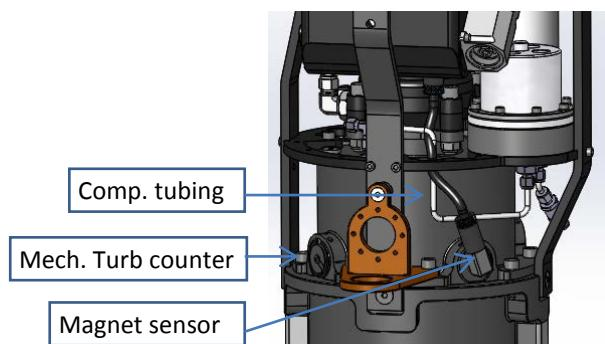
Figure 14: Detail components
