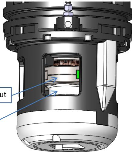
Figure 25: Concept with inductive transmission
