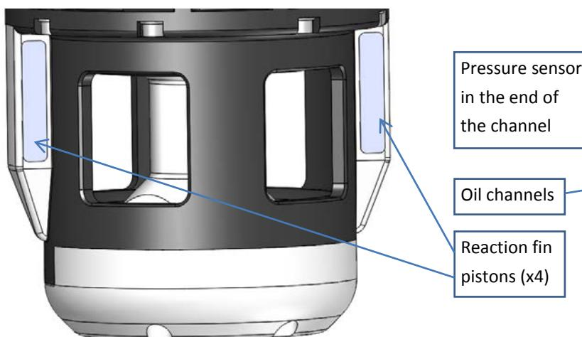
Figure 30: Reaction fin pressure sensor concept
