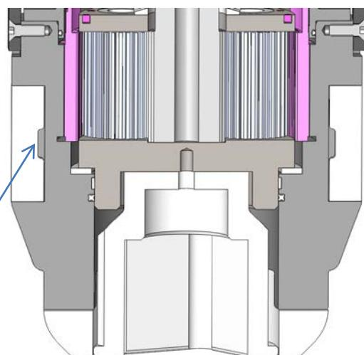
Figure 35: Section cut of strain gauges in reaction fins
