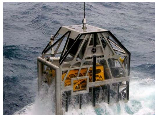
Picture 1: ROV deployed in a TMS (cage type) [6]
