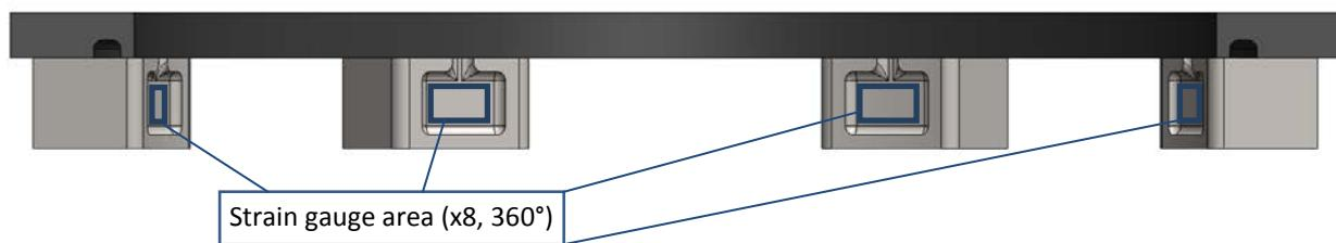
Figure 89: Section cut of strain gauge assembly
