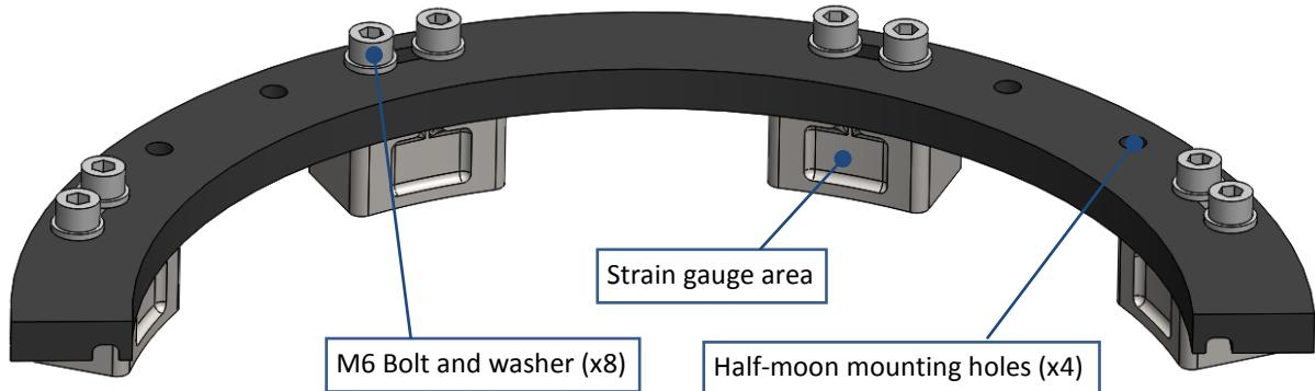
Figure 42: Transducer assembly, top view
