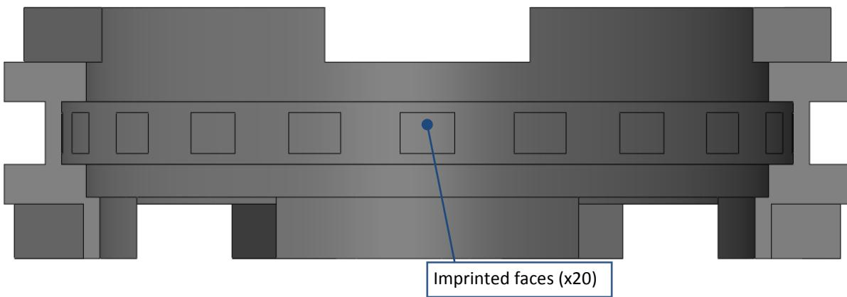
Figure 65: Transducer section cut showing SG area
