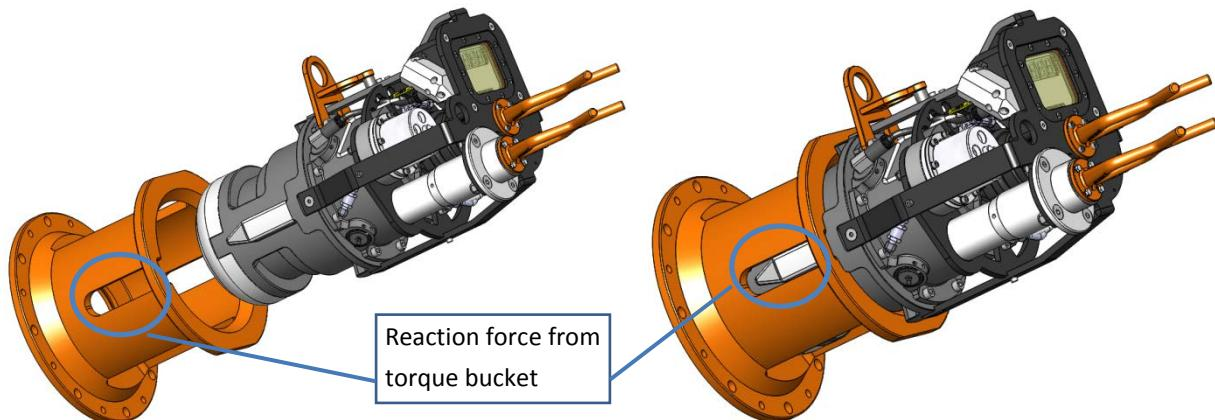
Figure 28: Existing tool undocked in interface bucket
