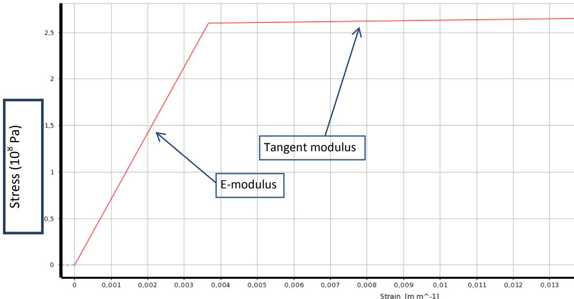
Figure 56: Bi-linear stress-strain curve for Alu 6082-T6 (from Ansys engineering data)
