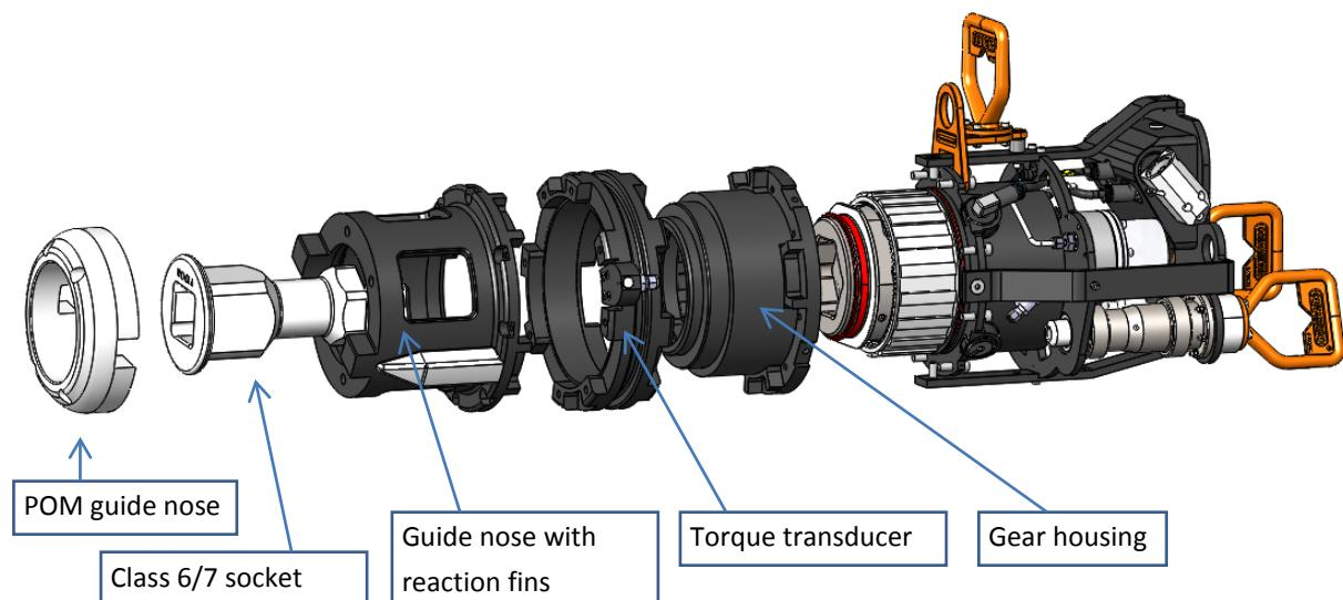
Figure 20: OAS concept design exploded view
