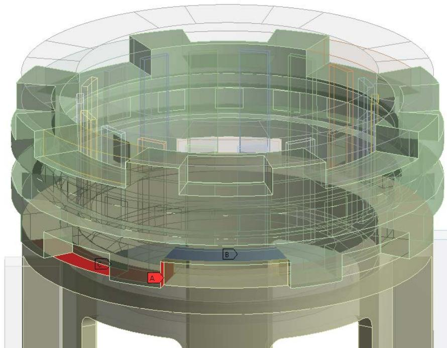
Figure 77: Tool guide and transducer contacts
