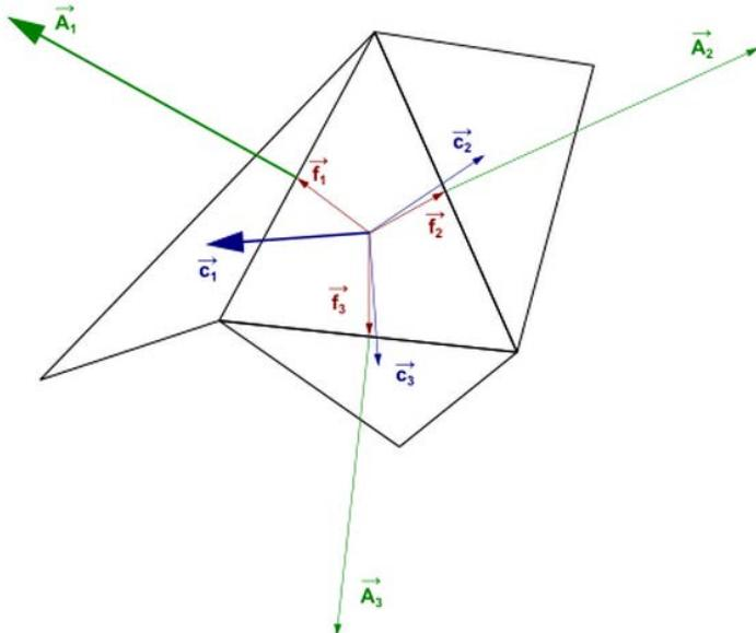
Figure 47: Vectors used to compute orthogonal quality [20]
