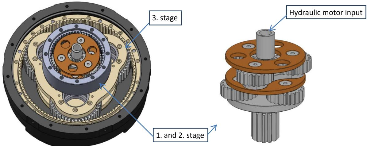
Figure 10: SAE TT gearbox design
