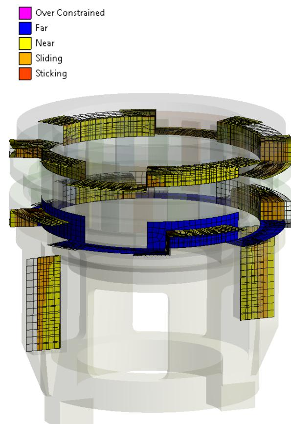
Figure 85: Final contacts for existing concept analysis
