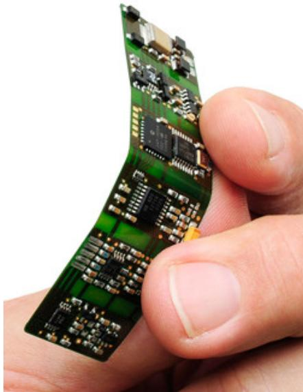
Picture 7: KMT flexible transmitter [16]
