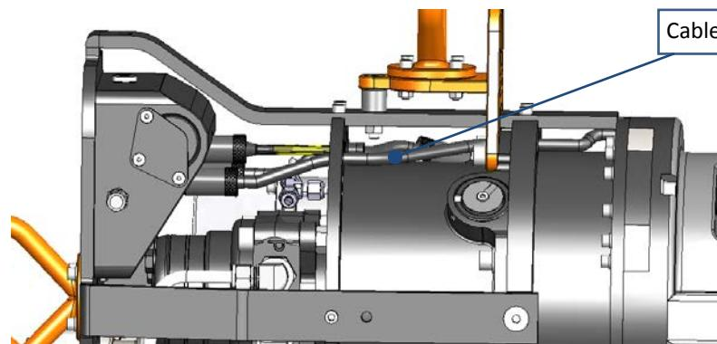
Figure 46: Cable routed to turn counter housing
