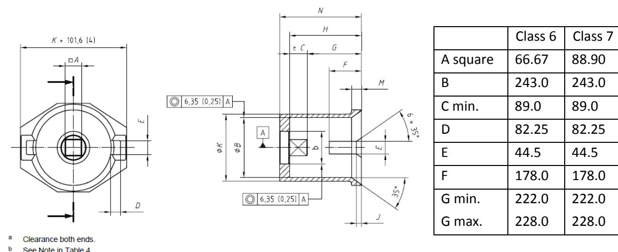
**Figure 6: Dimensions for receptacle (torque bucket)**
