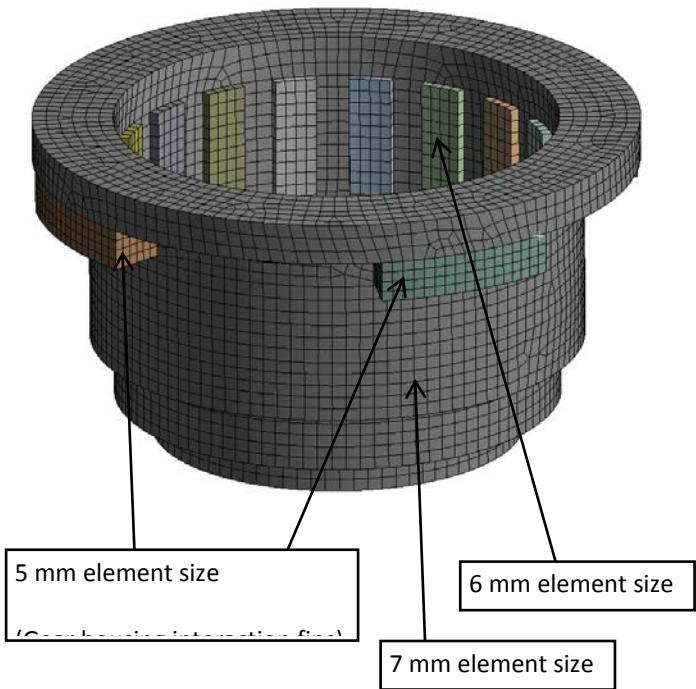
Figure 84: Gear housing multi-body part mesh
