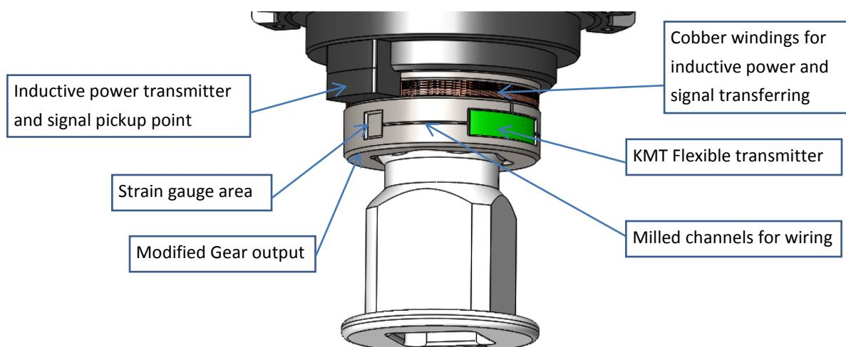
Figure 26: Customized KMT system on torque tool
