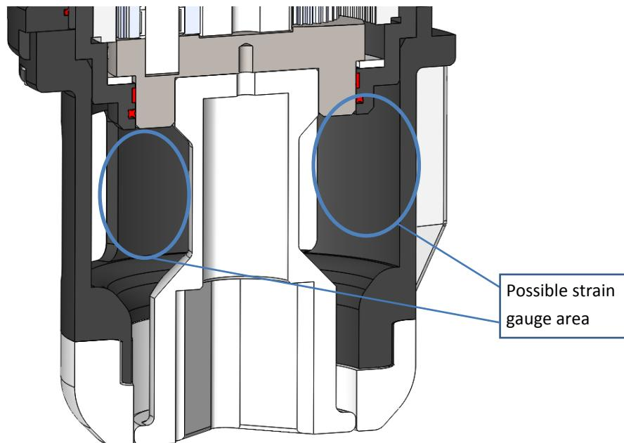
Figure 33: Strain gauge are close to reaction fins
