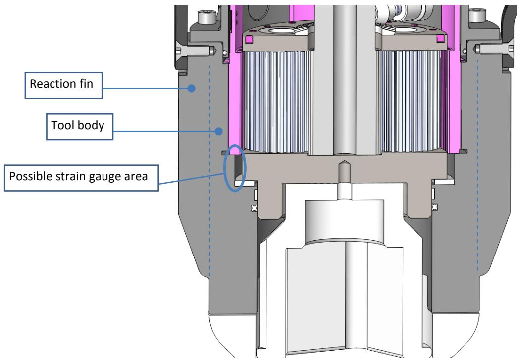
Figure 32: Strain gauges in reaction fins area on existing tool (section cut)
