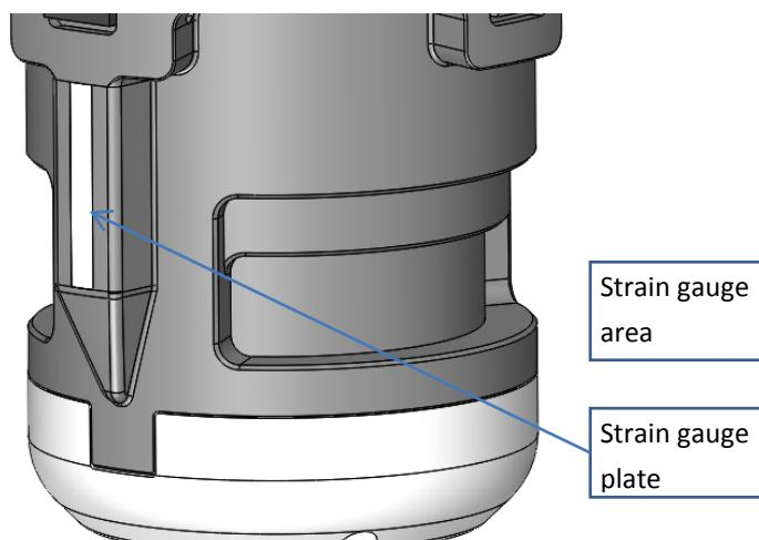
Figure 34: Strain gauges in reaction fins
