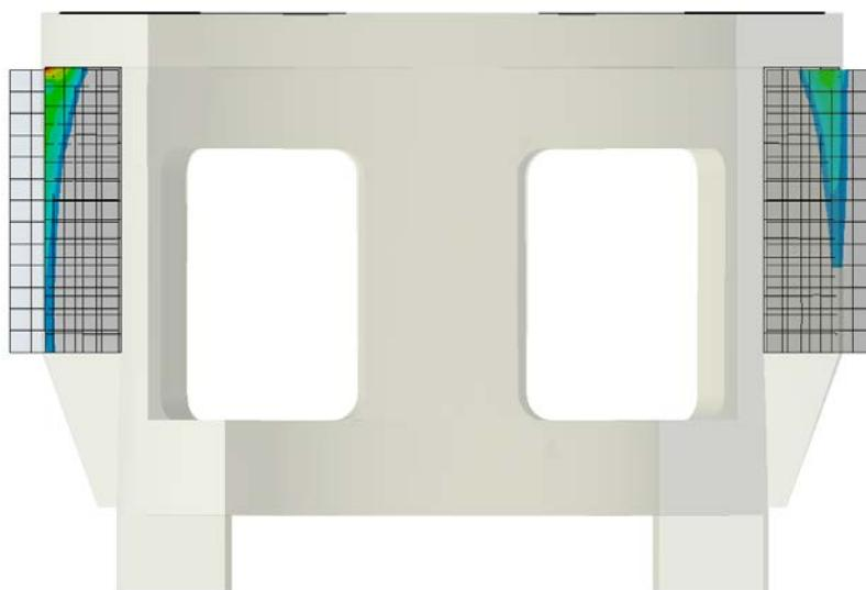
Figure 1: Pressure distribution on reaction fins
