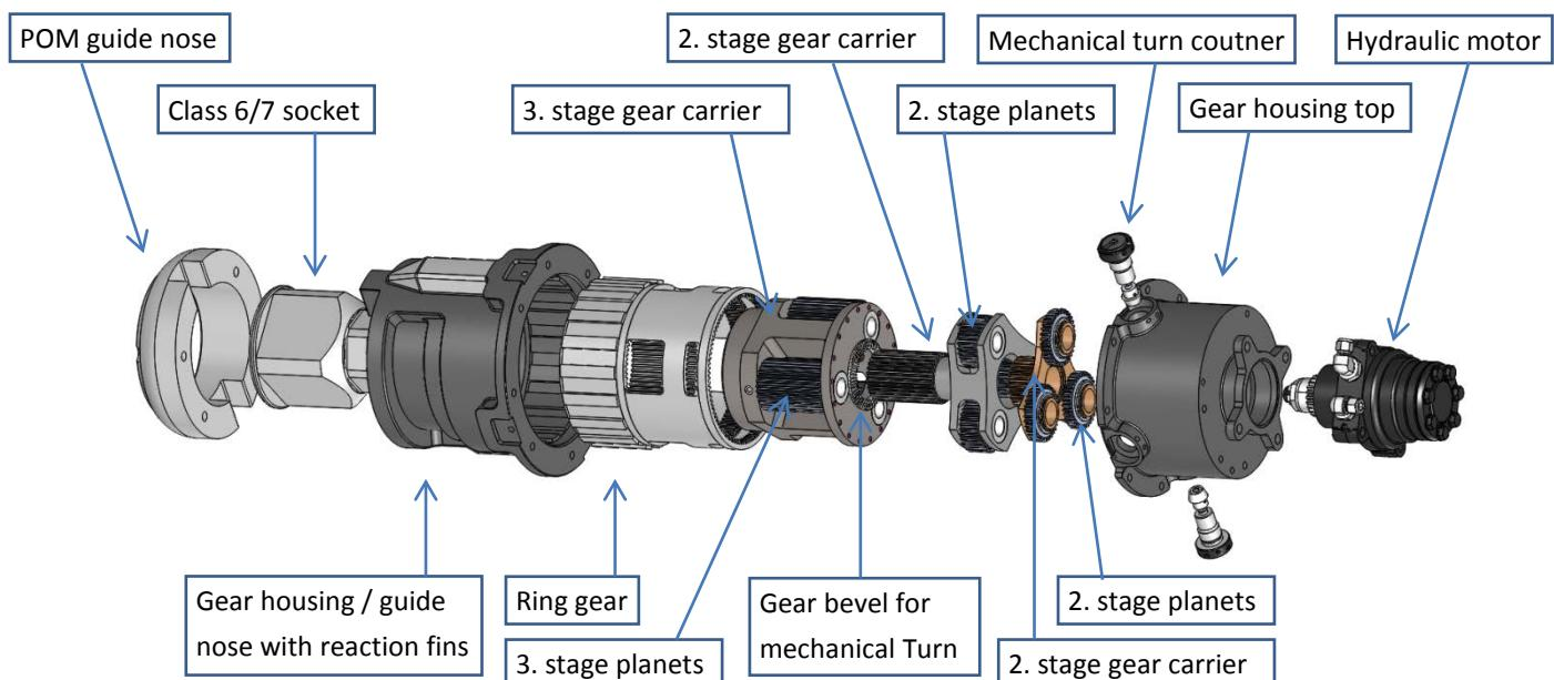
Figure 16: OAS TT exploded view
