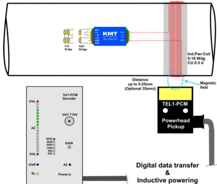
Figure 27: KMT block diagram [17]
