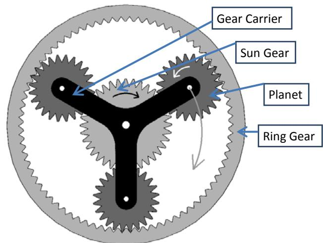
Figure 5: Planetary gear principle
