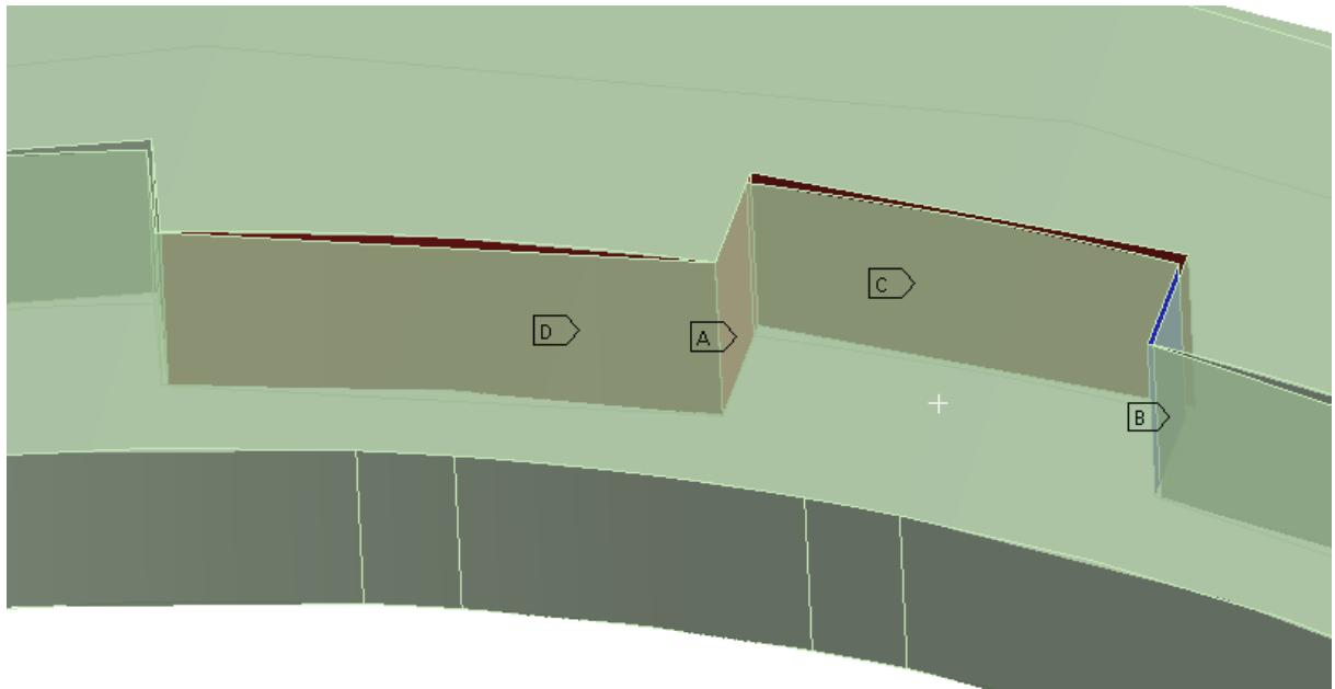
Figure 58: Frictionless contacts
