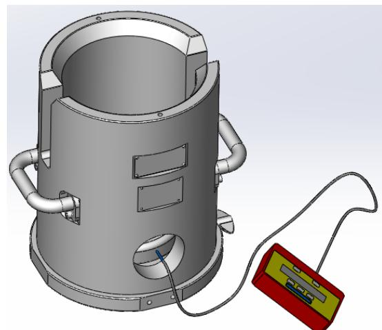
Figure 4: 3D model of Torque analyzer / calibration jig
