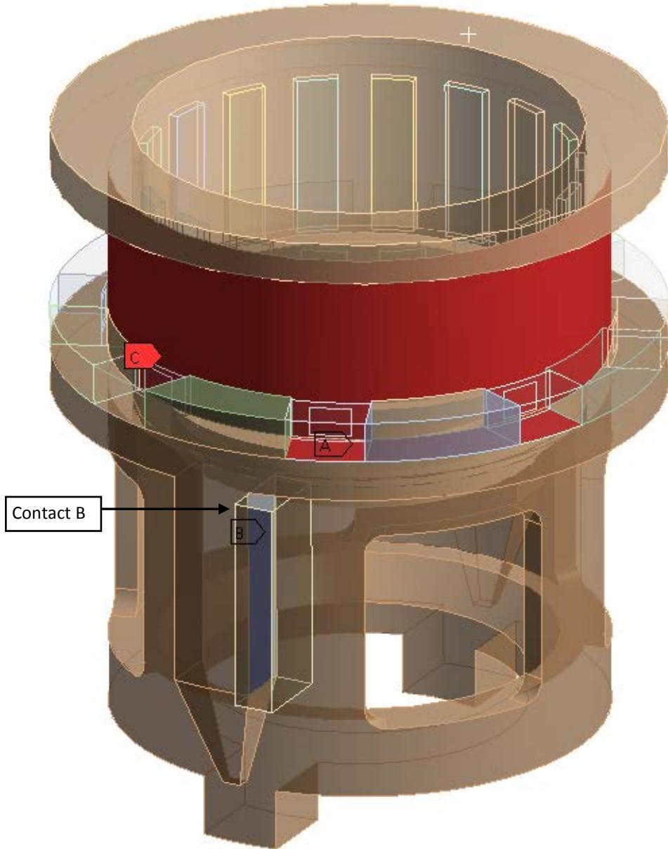
Figure 97: Contacts between gear housing and tool guide and tool guide and reaction plates
