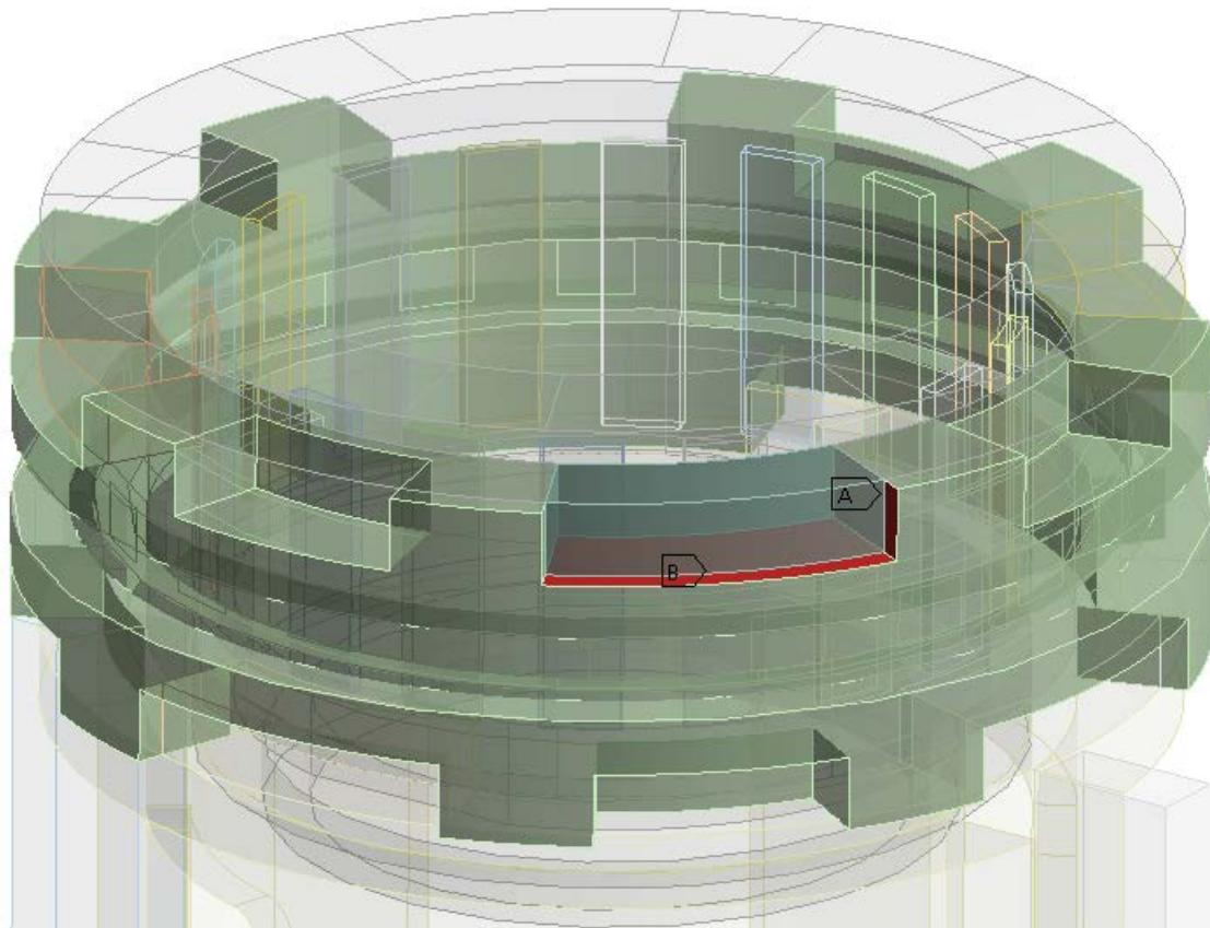
Figure 75: Gear housing and transducer contacts
