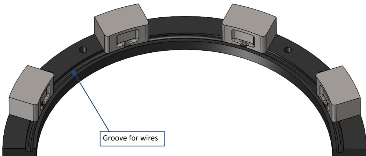
Figure 43: Transducer assembly, bottom view
