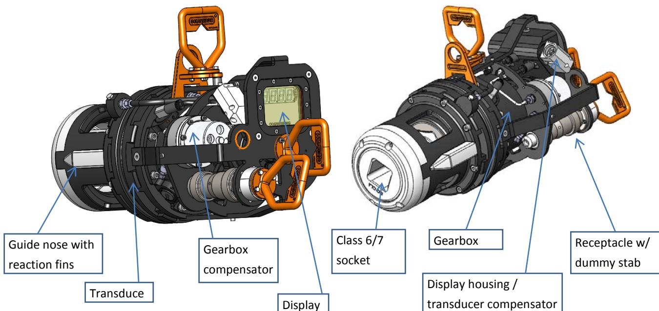
Figure 17: OAS concept design main components
