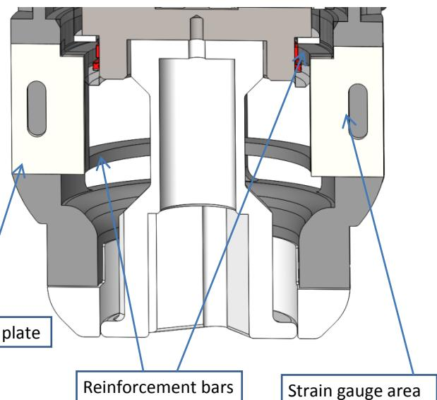
Figure 37: Section cut strain gauges in reaction fins
