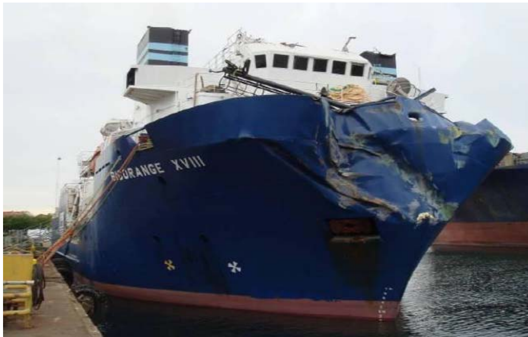
Figure 1-1 – Damage on Big Orange XVIII after the accident (Ref. /19)
