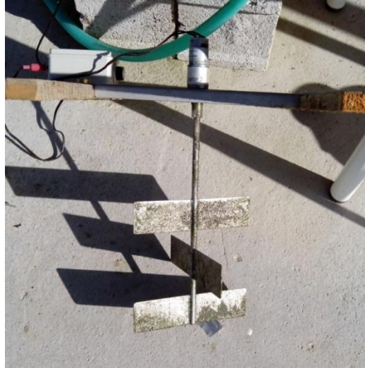
Figure 3.11 Paddle with motor attached on top and knob dial speed regulation on upper left.
