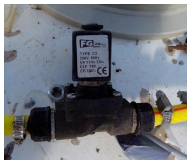
Figure 3.19 Side view of solenoid valve with specifications.
