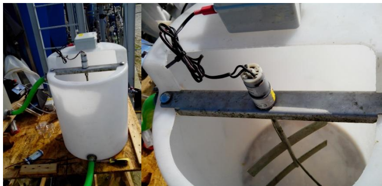
Figure 3.6: Left: 50 liters tank flocculator perspective with connections at the inlet and effluent. Right: 50 liters tank flocculator inside view with paddle, motor and knob dial attached.
