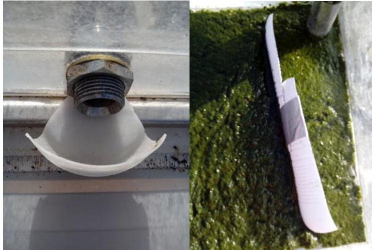
Figure 3.27 Left: First deflector made, designed for one single inlet. Right: Second deflector made, designed for 3 inlets.
