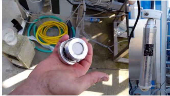
Figure 3.22: Left: Original SF500 water level sensor. Right: VEGAWELL52 water level sensor.
