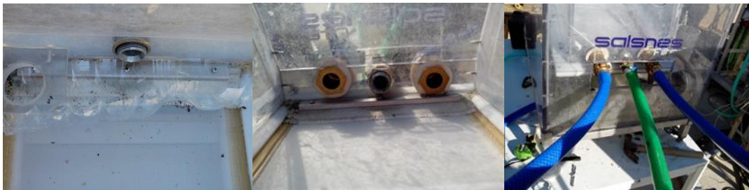
Figure 3.23: Left: 1 inlet SF500 (inside view). Middle: SF500 3 inlets (inside view). Right: SF500 3 inlets (outside view).
