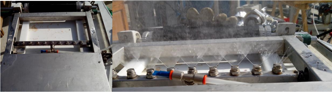
Figure 3.17 Left: Water knife set on frame. Right: Water knife working.
