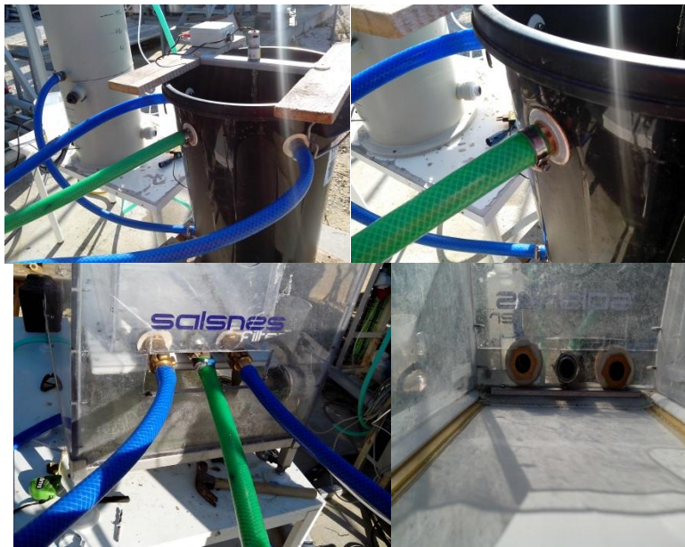
Figure 4.5: 20 Liters tank in combination with 100 Liters Pilot-scale Tank Flocculator.
