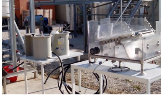
Figure 4.4: Configuration 1 - Pilot Scale Tank-Flocculator.
