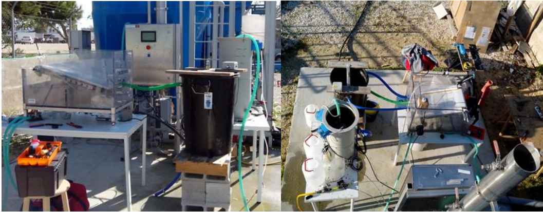
Figure 3.9: Left: Side view 100 Liters Pilot-scale Tank Flocculator Configuration. Right: aerial view.
