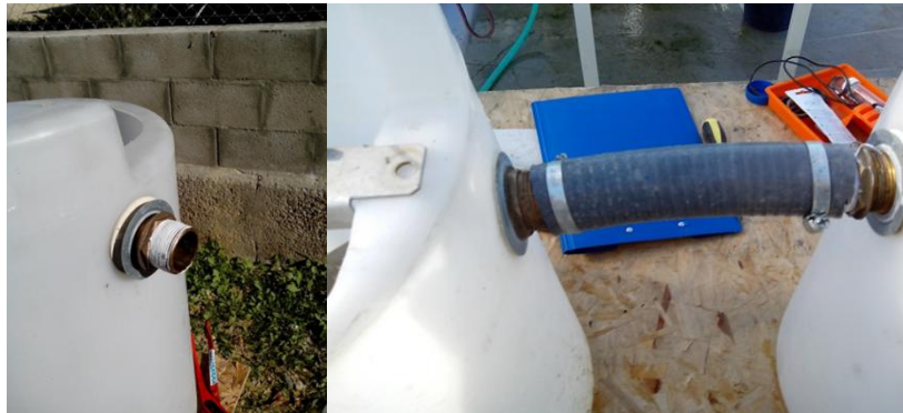
Figure 3.8: Up: Two 50 Liters Pilot-scale Tank Flocculator configuration. Left: 50 liters tank copper connection. Right: 50 mm diameter connection between both tanks.
