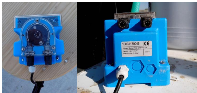
Figure 3.12 Left: Peristaltic pump. Right: Peristaltic pump specifications
