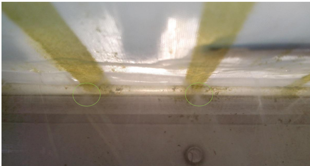
Figure 6.1: Actual crossing point of sprayed water by nozzle.
