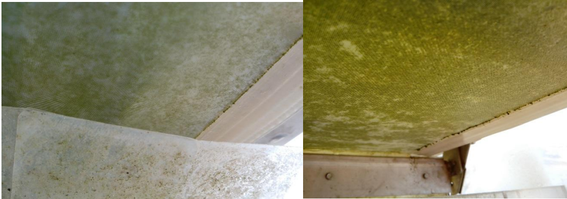
Figure 4.51: Up: Scraper working on a 350 µm mesh pore size, the green mesh is the result of algae particles not harvested. Left Below: Algae not harvested on 250 µm mesh. Right Below: Algae not harvested on 350 µm mesh.
