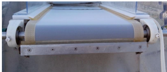
Figure 3.18 Plastic scraper set on filter.
