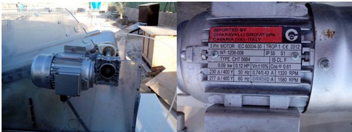
Figure 3.16 Left: Side view of motor attached to SF500, connected to a ruler to move the mesh. Right: Motor specification.
