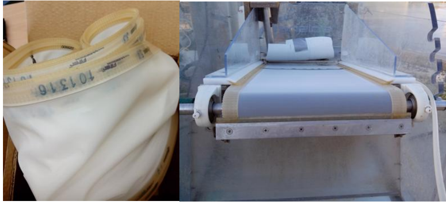
Figure 3.15 Left: Unpacked Salsnes Filter meshes. Right: Mesh set on SF500 frame.
