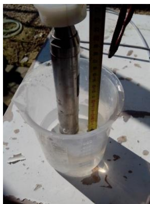
Figure 3.26: Water level sensor and meter partially submerged into water in order to calibrate it.
