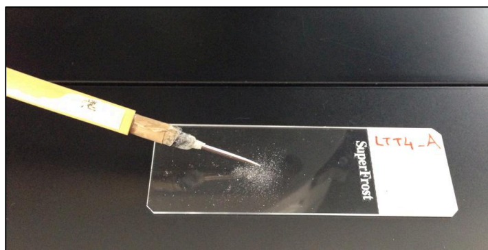
Figure 12: As whole rock analyses showed spectra strongly obscured by fluorescence, grains were scraped off from the sample and smeared out on a slide using a needle.
