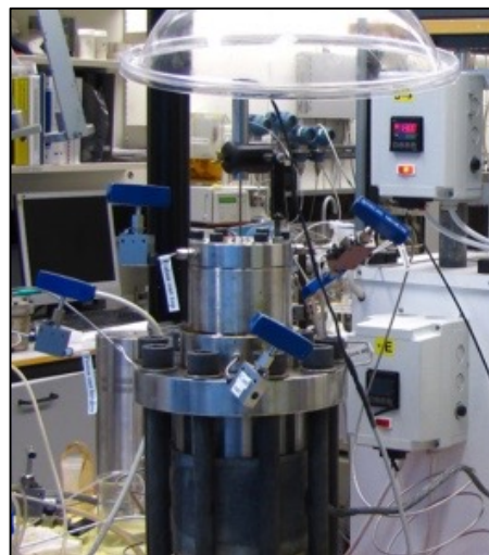
Figure 2: One of the triaxial cells in a laboratory at the University of Stavanger where the rocks were exposed to mechanical compression tests under reservoir conditions (University of Stavanger, 2013).
