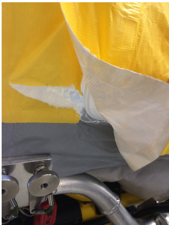
Figure 2 Ruptured suture after explosive decompression ( \Delta p 493hPa/7.15Psi).
