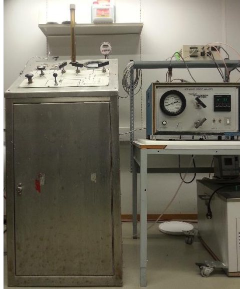
Figure 3.3 An Ultrasonic Cement Analyzer (UCA) with a pressure supplier.
