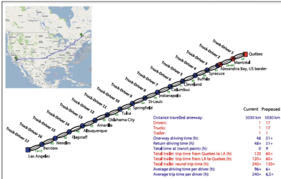
Figure 38: Contrasting current point-to-point transport and Physical Internet enabled distributed transport (Montreuil, 2011, p. 7)
