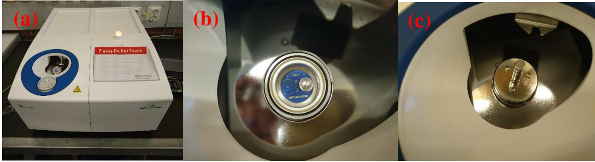
Figure 3.5: Differential Scanning Calorimetry: (a) the calorimeter; (b) the reference and the sample furnace chamber; (c) the furnace chamber with the furnace lid on.
