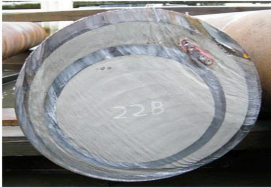
Figure 86 Pipe cemented inside casing with expandable cement and with attached control lines [26]
