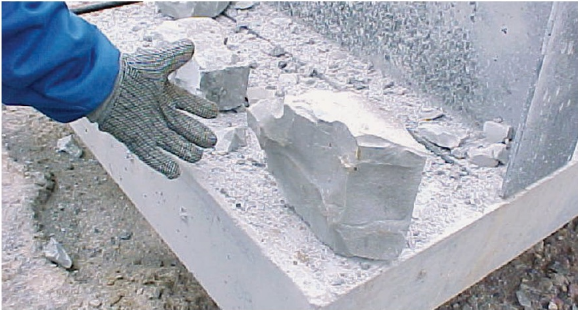
Figure 2: Thermal fracturing effect on cement [2]
