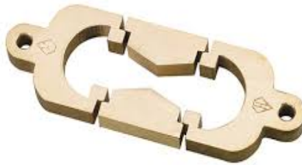
Figure 41 Briquette Mold used to measure tensile strength of cement [11]
