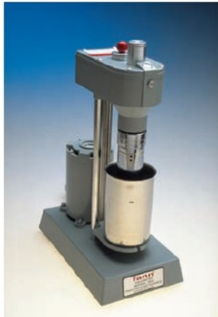
Figure 23: Couette-type rotational viscometer [2]
