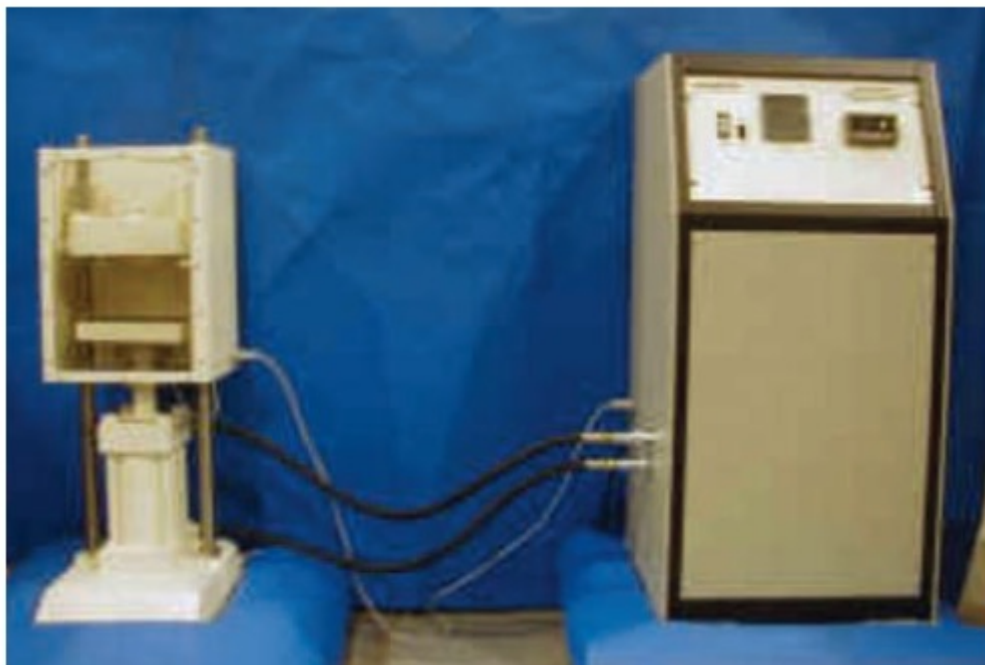
Figure 20: Hydraulic Press which measures the compressive strength of cement [2]
