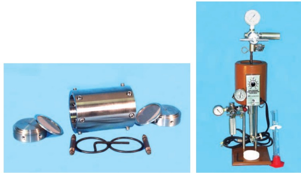
Figure 19: Filter Press with its components [2]
