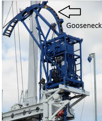
Figure 12 - Gooseneck mounted on an IH (modified version from [20])
