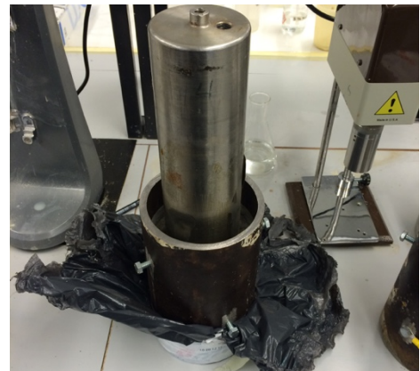
Figure 44: Tube number four with a metal tube inside for creating the desired cement thickness.
