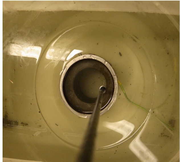
Figure 54: Test upset no. 4: The electrode rode was positioned into the cement wall, with a depth of 4,5 cm from the cement top. Fresh water was used.
