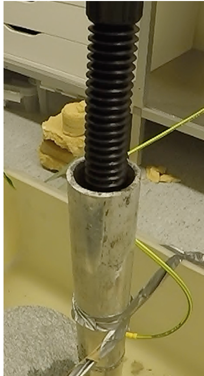
Figure 72: Setup 4. Aluminum Tube no. 1 was used with isolation A. Return electrode connected outside the tube and no water was added.
