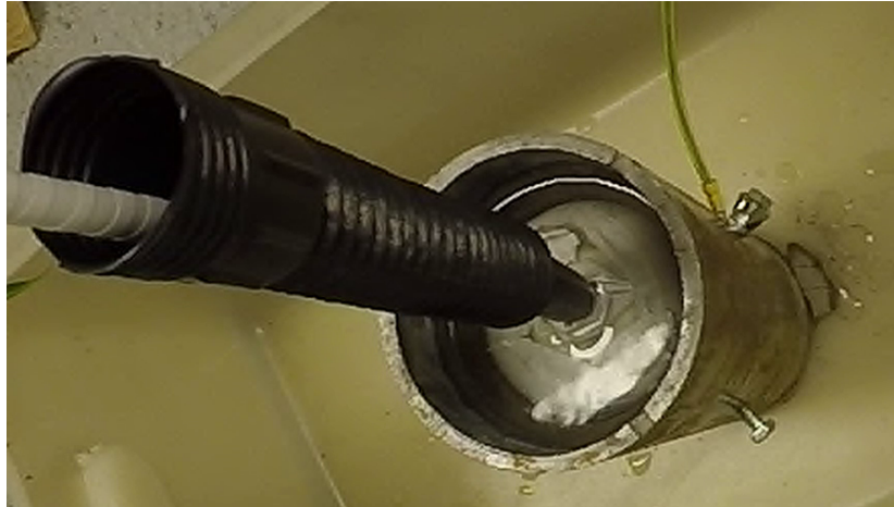
Figure 68: Setup 2. Tubing no. 2 with isolation A and B. Water was added to the top of cement.
