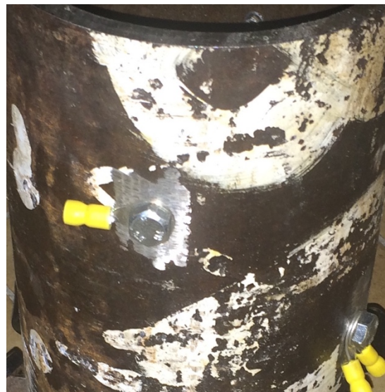
Figure 42: Scraped around the screw hole to get better connect between the wire and screws.
