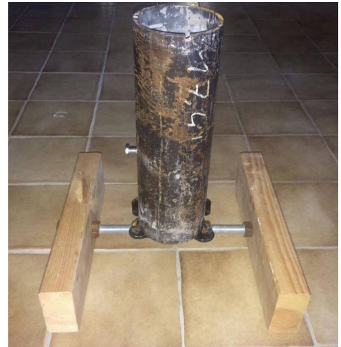
Figure 47: The test rig setup for holding the tubing in position during the experiments.
