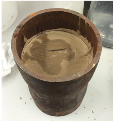
Figure 45: A Tube number 1 filled completely with cement and barite mix.
