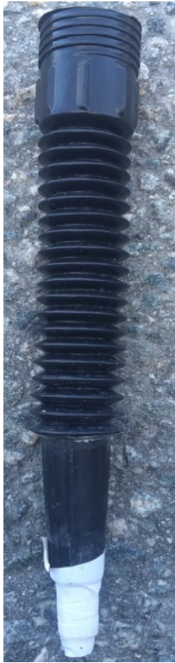
Figure 63 A: Isolater A, a funnel head from “Bilteam” was used to isolate and prevent the sparks jumping to the surface in the smaller sized tube.
