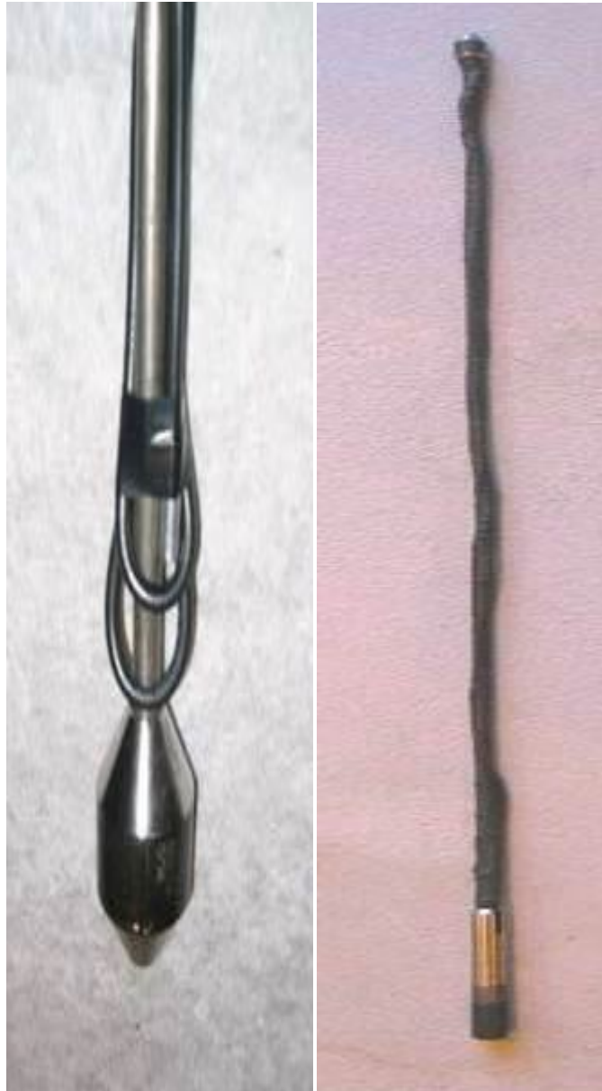
Figure 17: A detonating cord taped to a bar and a string shot (Statoil I. t.)
