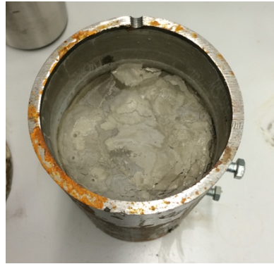
Figure 45: B Tube number 2 filled completely with cement.
