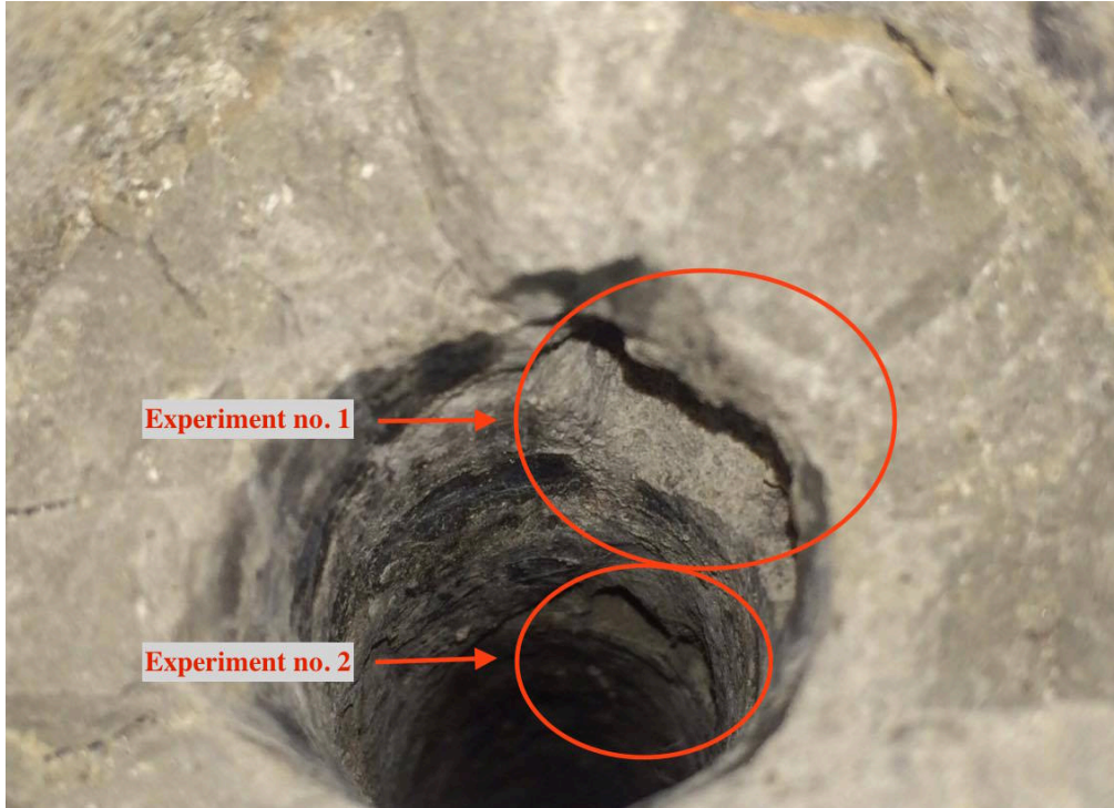
Figure 73: Test result from setup 4. To sparks from to different height was ignited and created two different shaped crater. Experiment no. 1 is shaped as a cone and experiment no. 2, two small elongated cone shaped.
