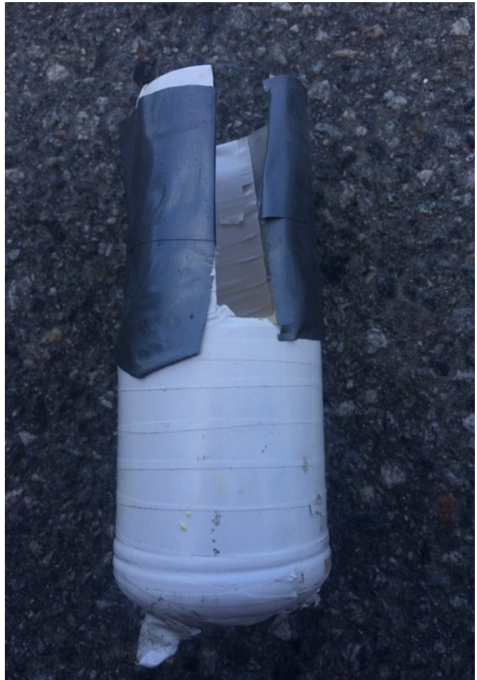
Figure 63 B: Isolater B, to prevent sparks jumping upwards to the surface and controlling the directions of the sparks by an opening in the isolation wall. A bottle was used, filled with isolation foam and surrounded with tape.
