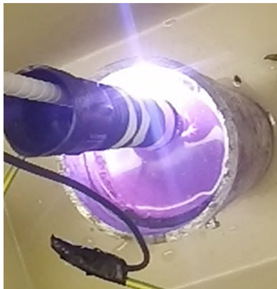
Figure 71: Test result from setup 3. The sparks created micro channels on the bottom of the tube and led to leakage.
