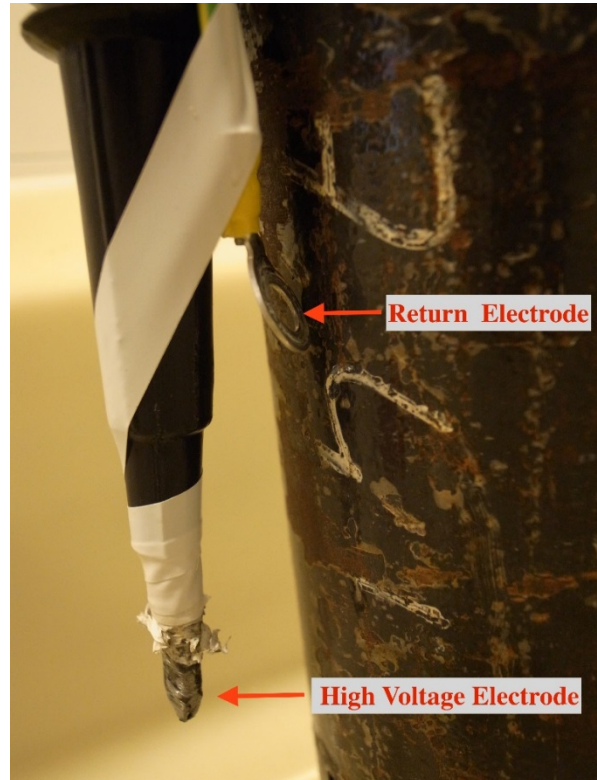
Figure 70: Setup 3. High voltage electrode and return electrode with a distance of 8,0 cm, placed inside the tube with fresh water.
