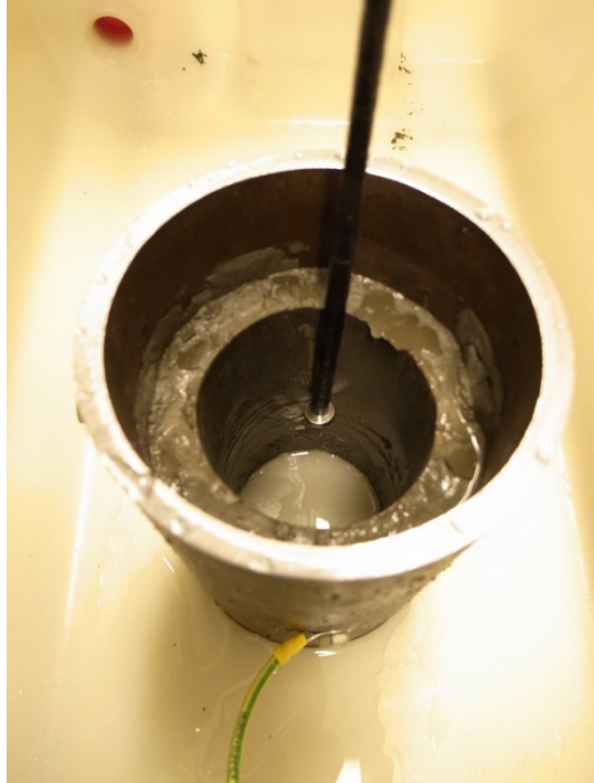
Figure 58: Setup 5: The electrode was positioned into the cement wall, with a depth of 4,5 cm from the cement top. No water was used.
