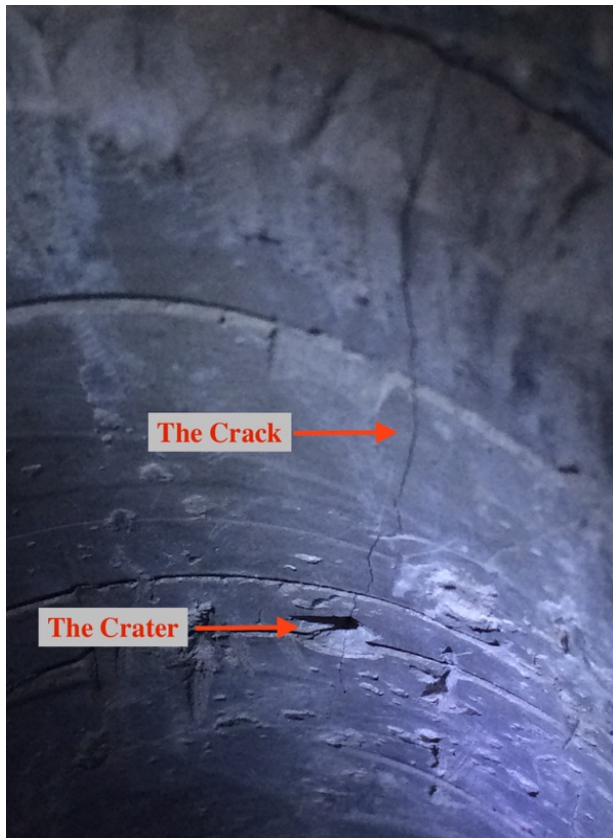
Figure 66: Test result from setup 1. The spark created a crater and fractured the cement all the way to the top.
