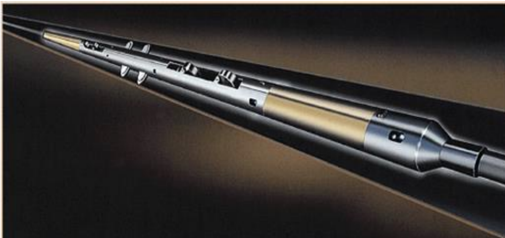
Figure 25: Well tractor whose wheels are released against the wellbore ( (Nergaard & Grimholt, 2010))
