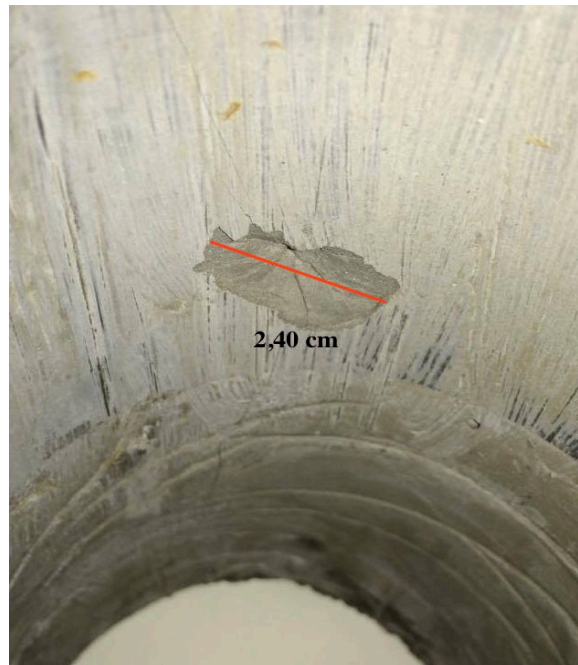
Figure 55: Test result no. 4: Damage to cement due to the sparks and shock wave. The diameter of the damaged zone is 2,40 cm.
