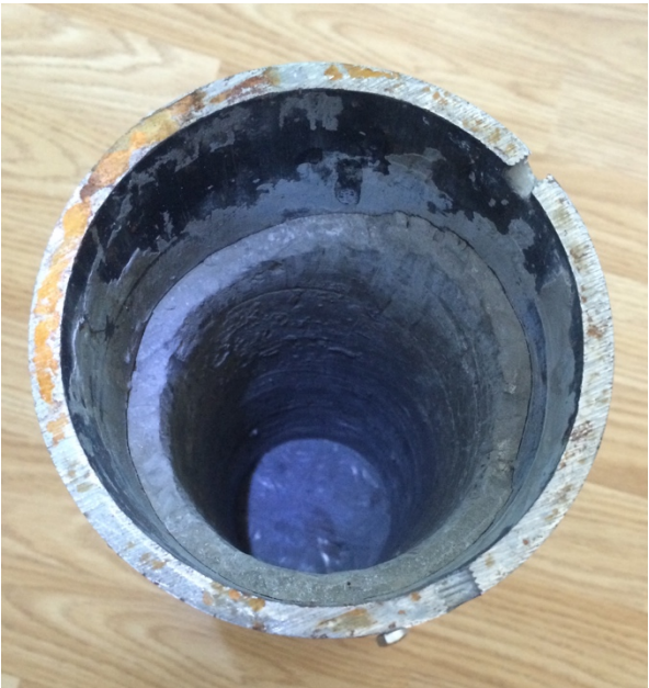
Figure 64 B: Tubing no. 2 with an inner diameter of 10,2 cm and a cement thickness of 2,0 cm. Closed ended with cement.
