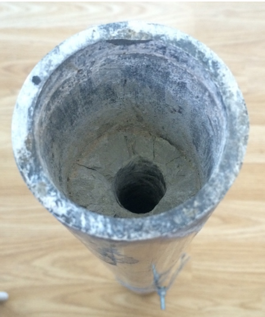
Figure 64 A: Tubing no. 1 with inner diameter of 5,1 cm and a cement thickness of 2,0 cm. Open ended.
