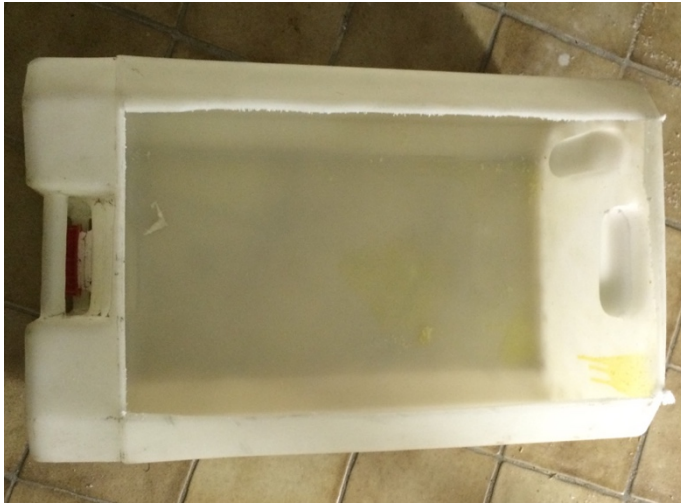
Figure 46: Plastic container for putting the test rig setup inside and holding the water in place.
