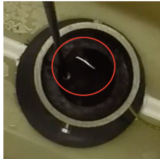
Figure 61 B: The spark goes towards the cement top and causes some damage.
