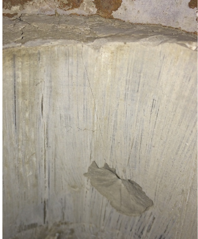
Figure 57: Test result no. 4: The crack has propagated up to the top of the cement. The picture is taken from above of the tube.
