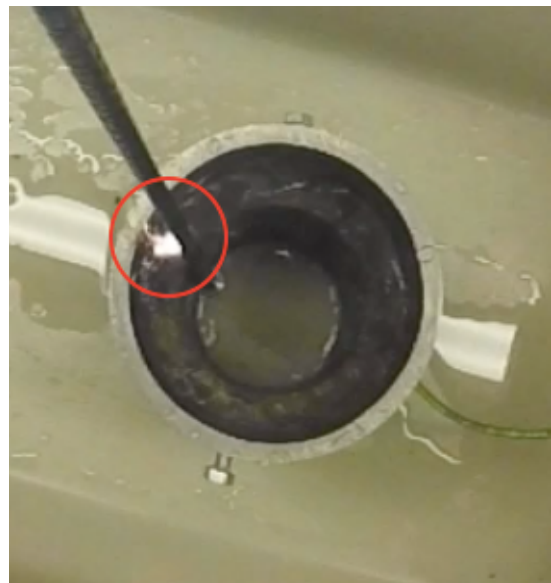
Figure 59: Test result no. 5: The sparks went to the top of the tubing as shown in the picture.
