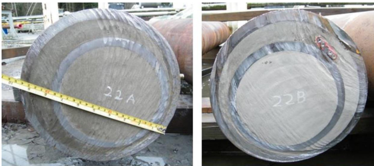
Figure 54 – Assemblies with expandable cement cut crosswise through. Assembly without control lines to the left and with control lines to the right. Perfect displacement around the control lines. (44)
