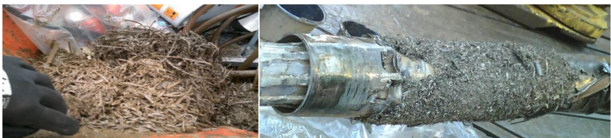
Figure 28 – Swarf from milling operation
