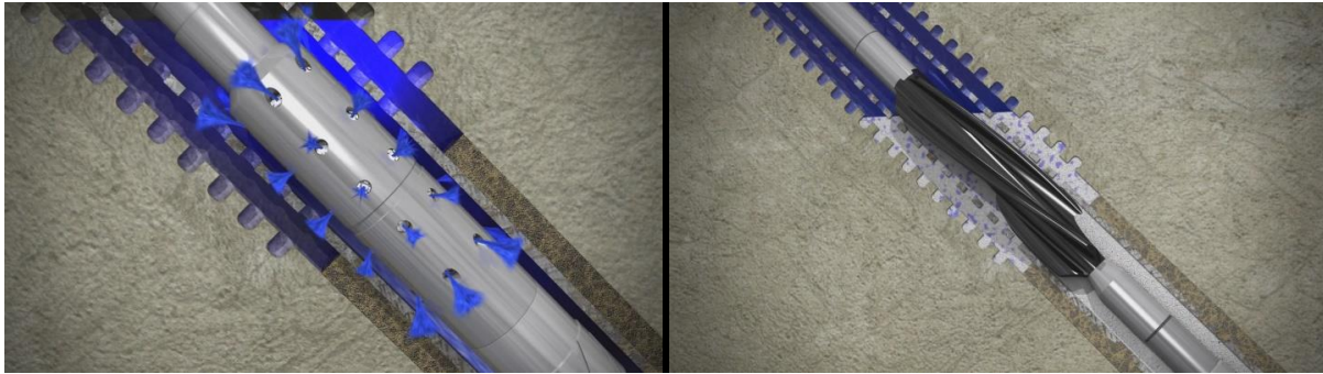
Figure 39 – (Left) HydraHemera Jetting tool injecting spacer fluid. (Right) HydraArchimedes forcing cement into the annuli (34)
