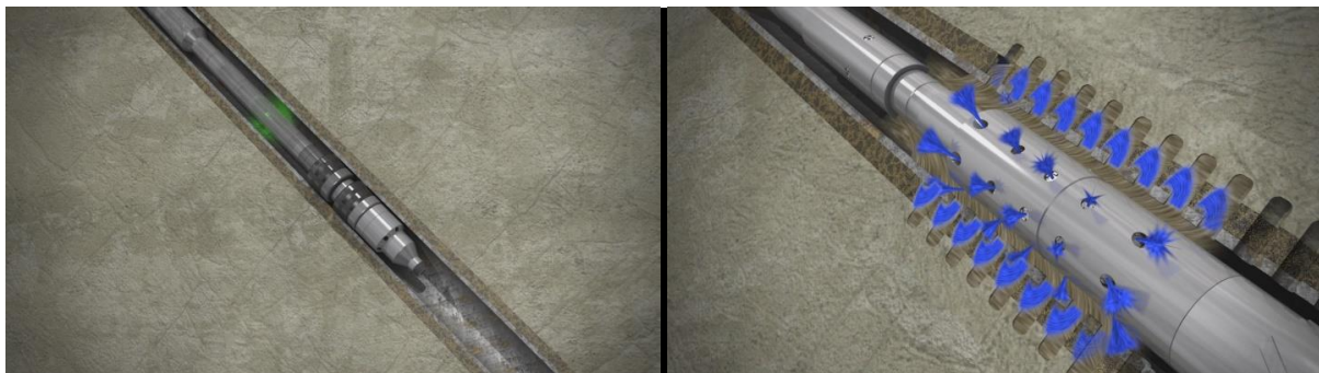
Figure 38 – (Left) Internal Cement foundation (ICF). (Right) HydraHemera Jetting tool (34)
