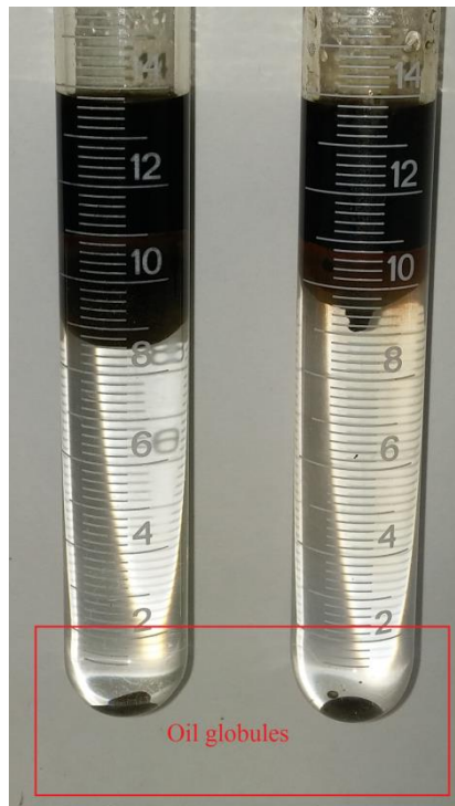
Figure 31: After N-decane had been added to remove STO #2.
