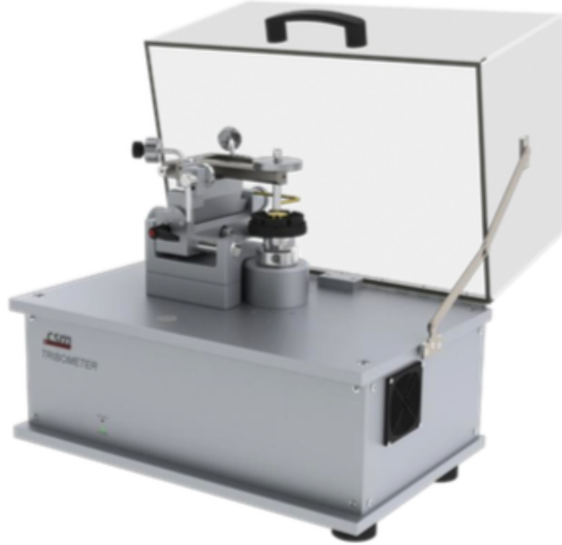
Figure 42: Displays the tribometer used in the experiments to solve the main idea of this thesis. Determination of local friction factor in wellbore Instruments [2010].
