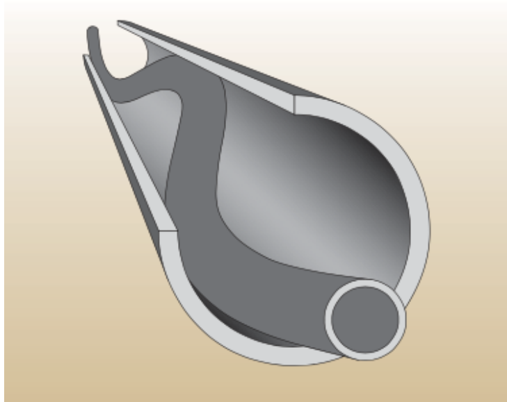
Figure 22: Sinusoidal Buckling. This is the first order of buckling when a load is applied Bennetzen et al. [2010].
