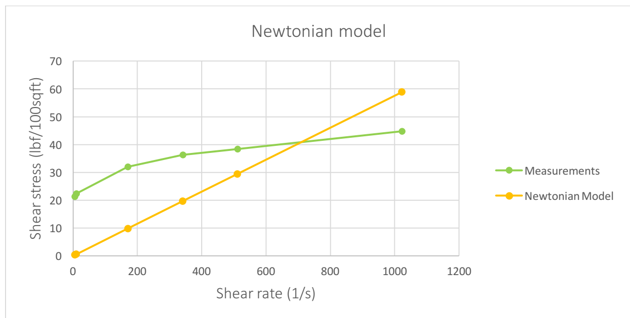
Figure 3.5: An illustration of the Newtonian fluid model
