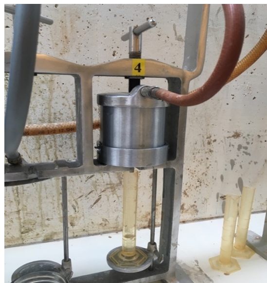
Figure 4.2: Filtrate loss measurement with an API Filter press
