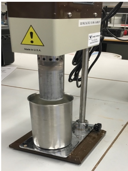
Figure 4.1 Fann-35 Viscometer used for readings
