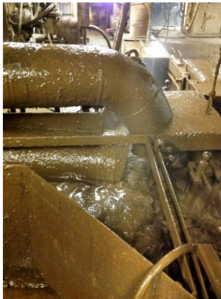
Figure 19: Header box at the semi-submersible drilling rig showing the turbulent flow created by the air blower.
