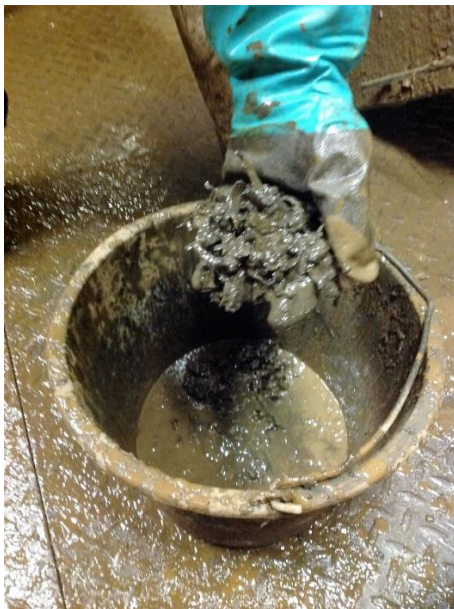
Figure 24: Ditch magnet sample taken from EZ-Clean ditch magnet at the semi-submersible drilling rig.
