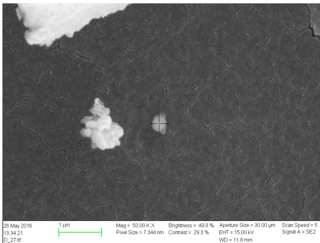
Figure 36: The investigated area of the magnetic particle marked with a cross. Only a small spot was investigated.
