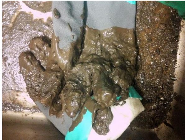
Figure 23: Magnetic waste taken from M.A.P.S ditch magnet on the jack-up drilling rig.
