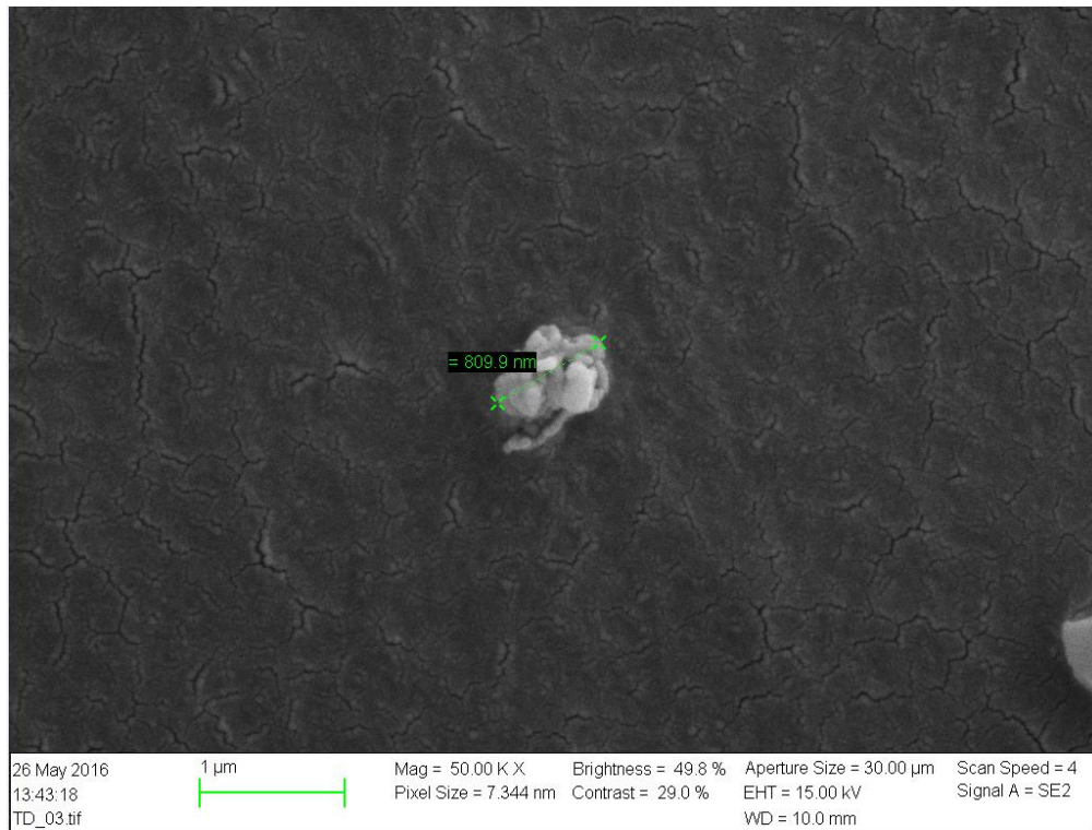
Figure 32: Magnetic particle collected by the EZ-Clean ditch magnet
