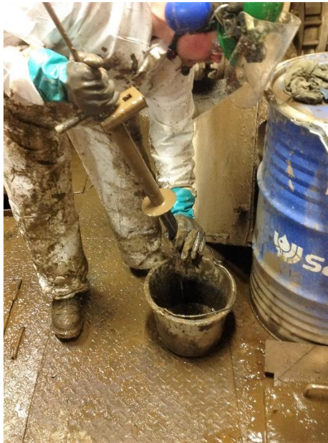
Figure 8: Cleaning of EZ-Clean ditch magnet. Picture taken at the semi-submersible drilling rig.
