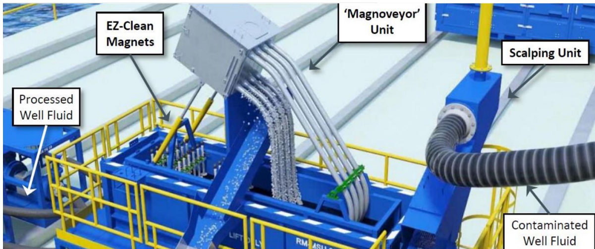
Figure 22: Swarf Handling System by Romar International [25].
