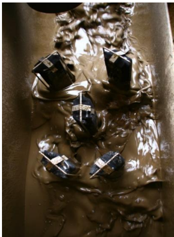
Figure 11: Magnetic Mud Filter™ installation [22].
