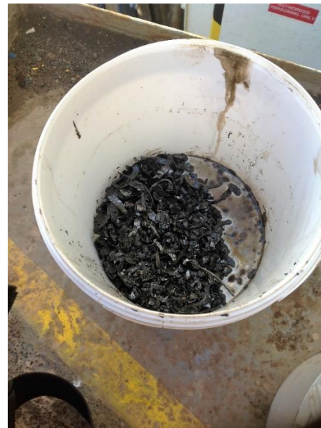
Figure 25: Ditch magnet sample from the semi-submersible drilling rig cleaned with base oil and sieved with a 2mm mesh size.
